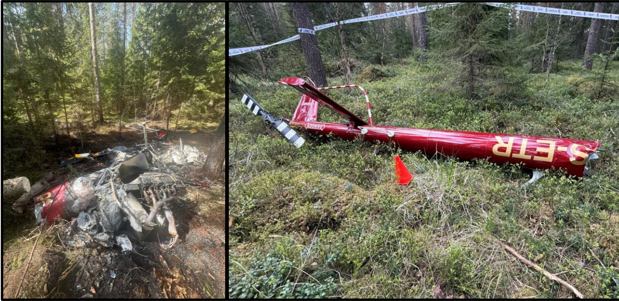
Figure 2. Wreckage of ES-ETR. The fuselage with a section of the main rotor system (left), and the tail boom (right). The marking cone was placed by investigators. (Photo: SIAF)
