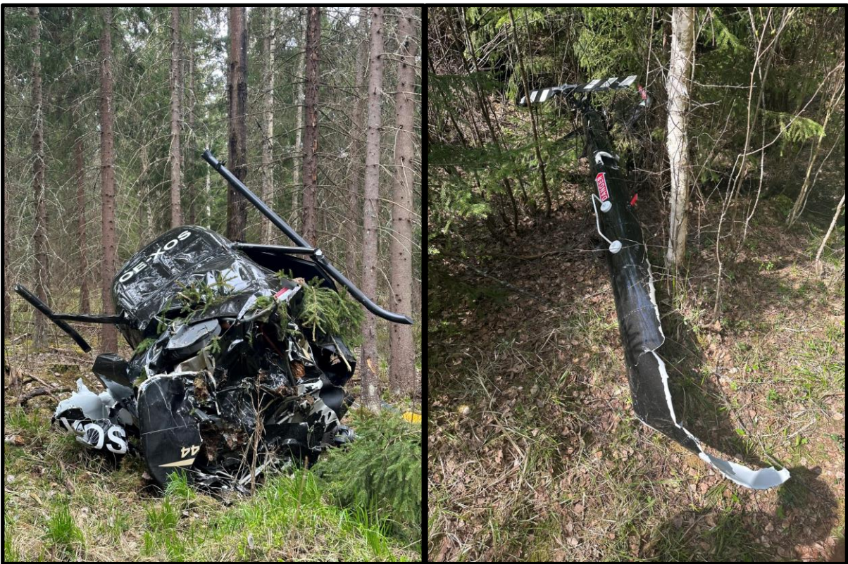
Figure 3. Wreckage of OE-XOS. The fuselage (left), and the tail boom (right). (Photo: SIAF)
