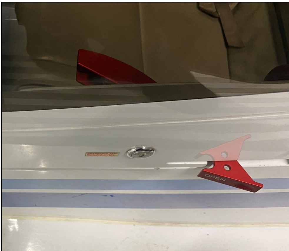
Figure 11. The external and internal door handle in the position that triggers the door warning. (Photo: SIAF)
