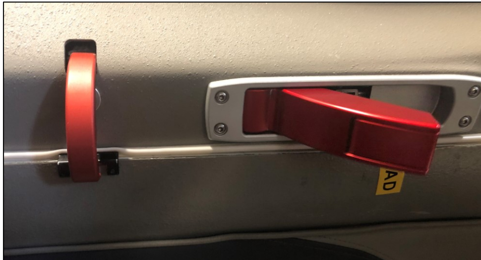
Figure 7. The internal door handle (right) in a partially open position and the safety catch (left). (Photo: SIAF)
