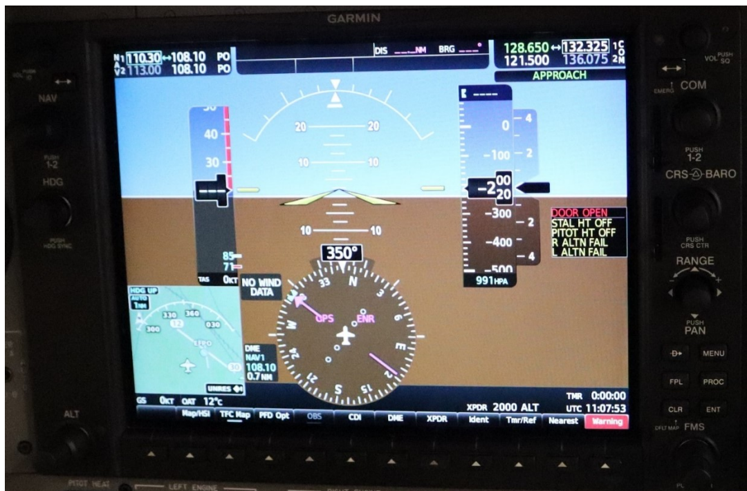
Figure 5. A PFD view after a door warning. Warnings, cautions and advisories appear in the notification window on the right. When a warning is triggered, “Warning” flashes on red background in the bottom right corner and an aural warning sounds. (Photo: SIAF)
