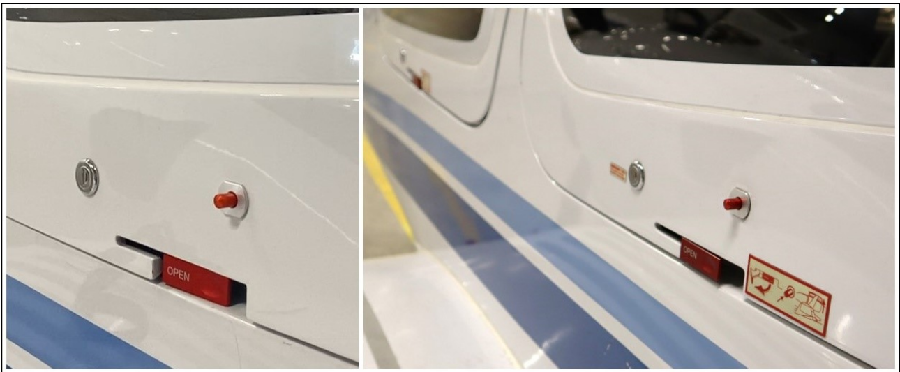
Figure 12. The fully locked position of the external handle appeared different in the two airplanes. Left (OH-DAN with a new door): the handle is recessed by approximately 8 mm. Right (OH-DAM): the handle is slightly proud of the door frame. (Photos: SIAF)
