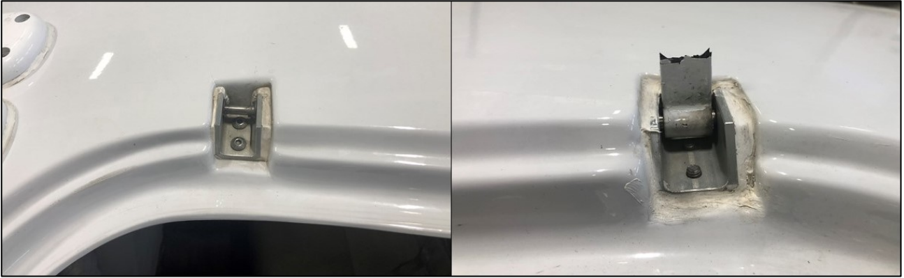
Figure 2. Damaged door hinge assemblies. (Photos: SIAF)
