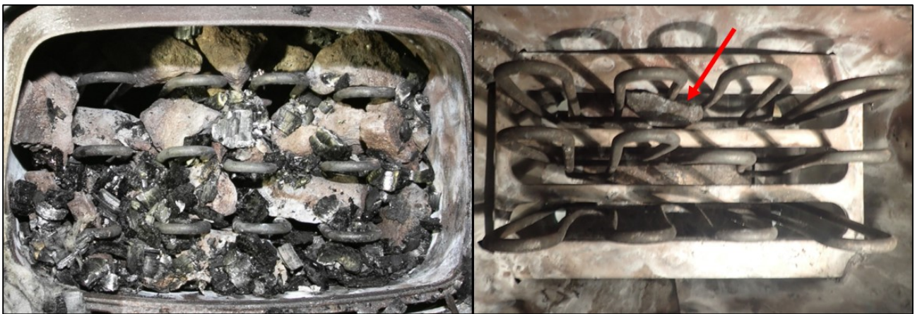
Figure 18. On the left, a photo taken during the site investigation, in which about two layers of stones had already been removed from the heater. The stones were in a tight contact both with each other and with the electrical heating elements and the casing of the stone space. The charred pieces of wood had fallen on top of the heater during the fire. On the right, the photo taken after the stones were removed shows one tightly wedged stone that had pressed the heating element against the heater's metal structure. (Photo on the left: the police; Photo on the right: Safety Investigation Authority, Finland)
