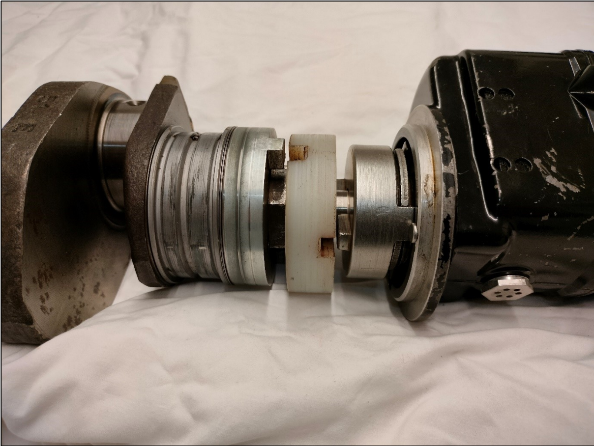
Figure 12. The rear end of the crankshaft, the magneto, and the magneto drive coupling. (Photo: SIAF)
