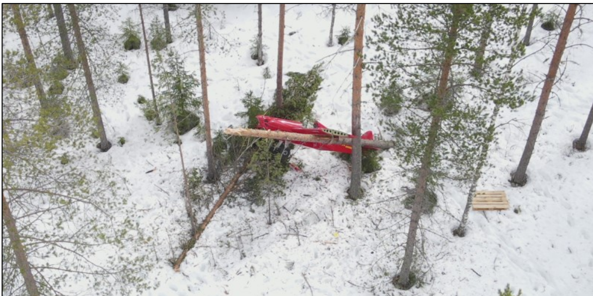
Figure 6. The impact severed the pine tree on which the airplane came to rest. The pallet was brought to the site after the accident. (Photo: Police)
