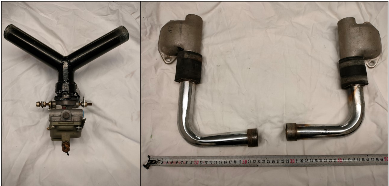
Figure 3. On the left: the carburetor and the Y-junction of the inlet ducting. On the right: inlet ducts leading to the cylinder heads. (Photo: SIAF)
