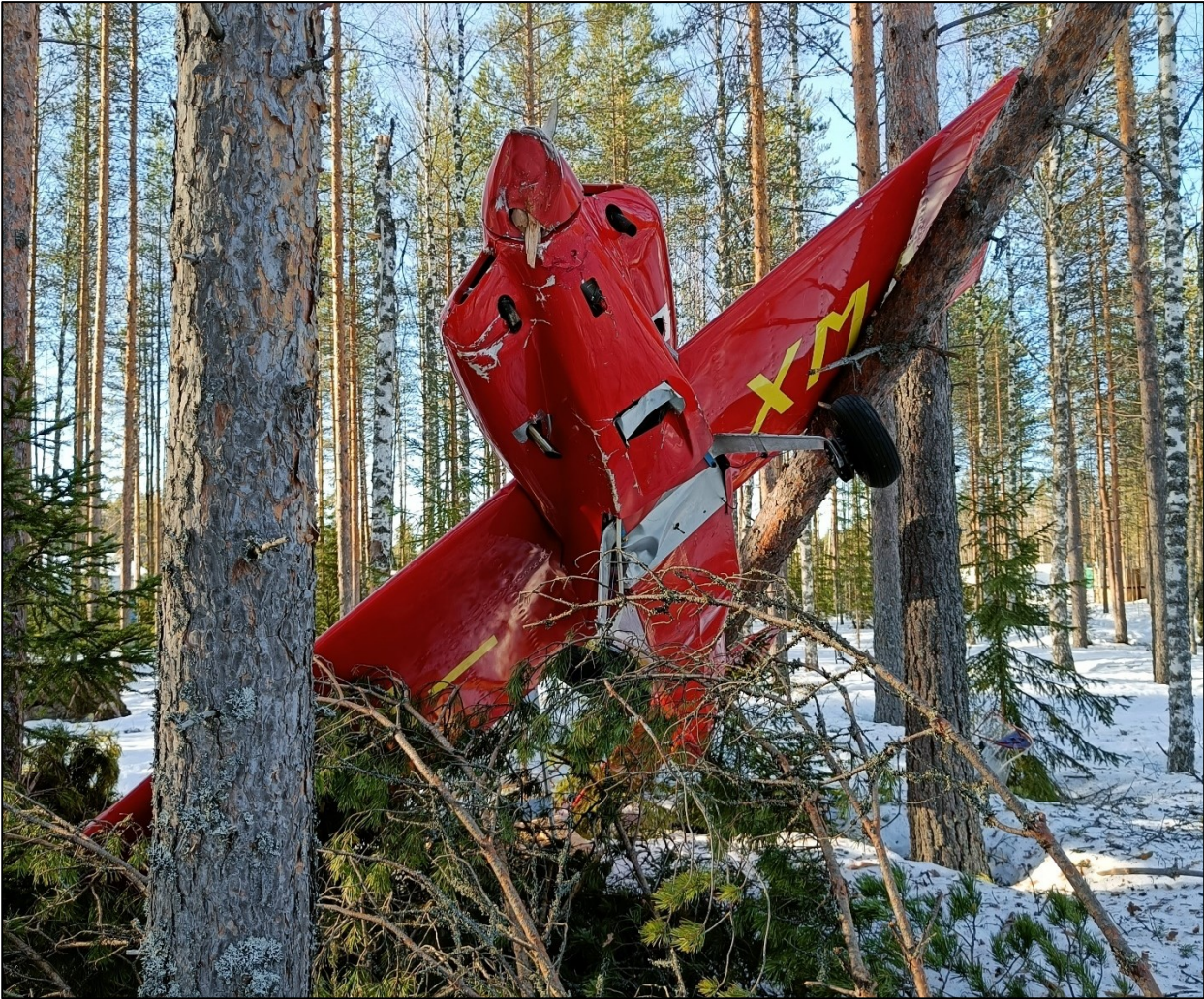
Figure 7. The airplane came to rest supported by a severed tree. The propeller blades broke off near the root, and the spinner exhibited denting. The cowling was impact-damaged. The forward right-hand exhaust was bent. (Photo: SIAF)
