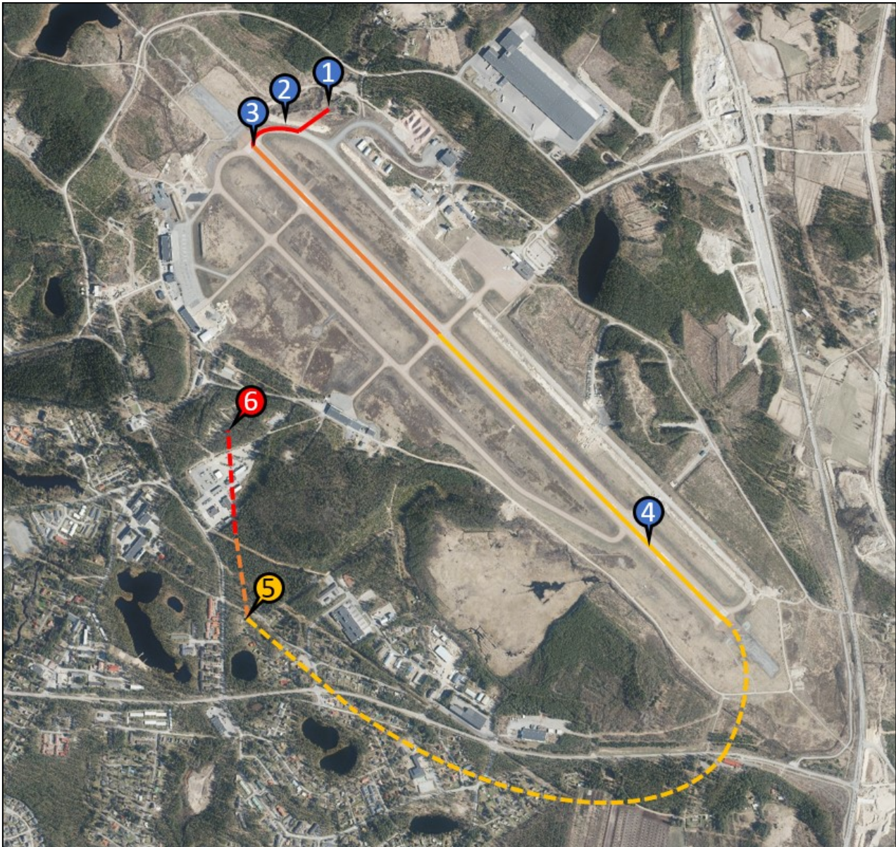
Figure 1. The estimated flight track of OH-XMA. Key: 1. Initial radio call at 1919 h. 2. Reports at holding point A at 1922 h. 3. Reports takeoff from runway 12 at 1924 h. 4. Reports right turn at 1925 h, estimated position. 5. Engine cuts out, estimated position. 6. Accident site. (Photo: Orthoimage ©National Land Survey of Finland 2/2023, annotated by SIAF)
