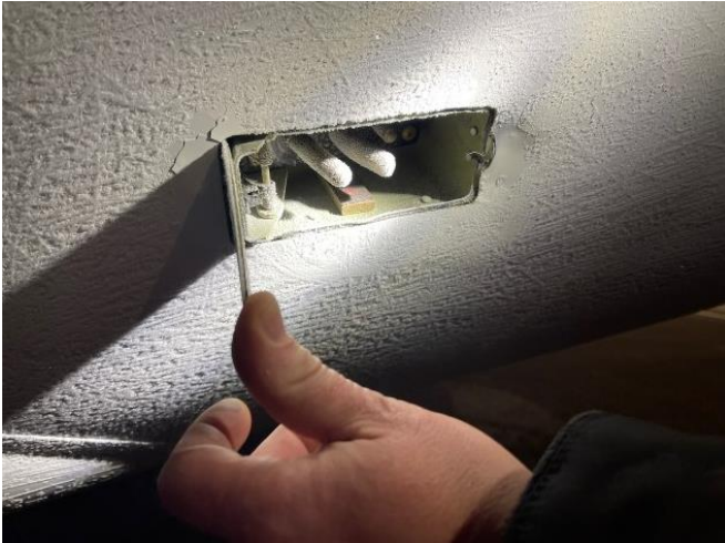
Figure 5 The GPU receptacle pins exhibited bending, and the fuselage skin around the receptacle was deformed under cable tension. (Photo: SIAF)
