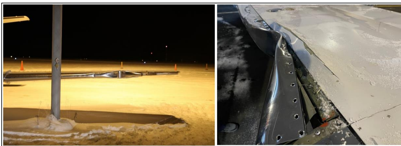
Figure 4 The dent in the left wing leading edge extends all the way to the wing spar. (Photos: SIAF)
