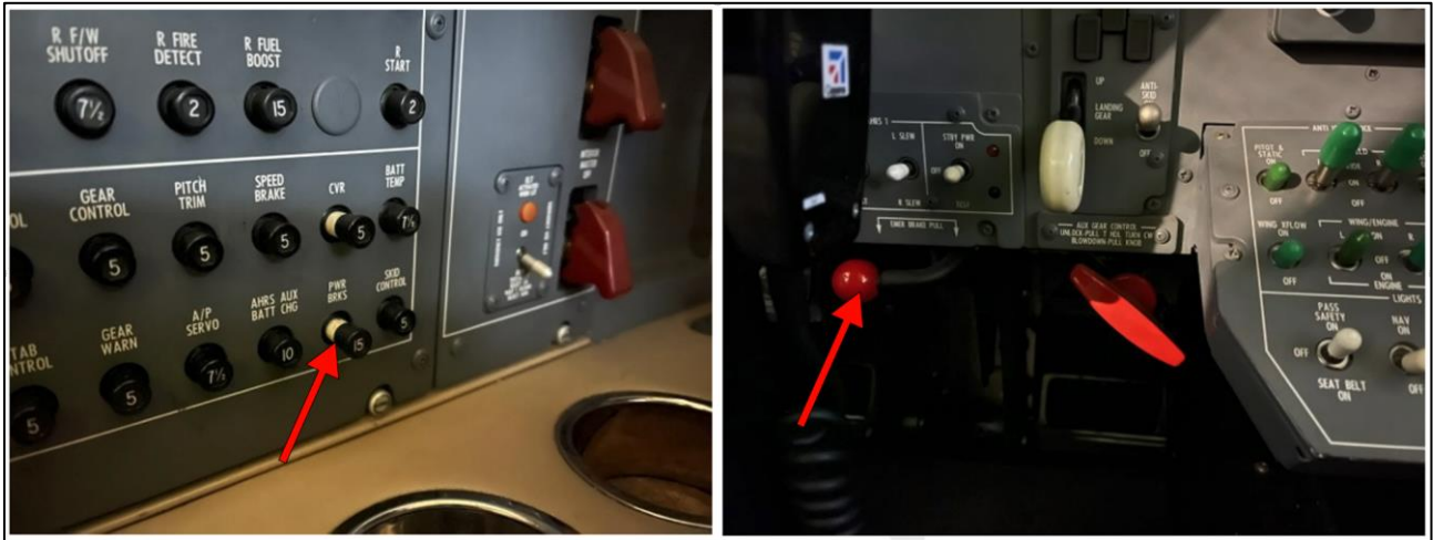
Figure 6 Left: The circuit breaker panel next to the left seat. The arrow points at the tripped brake system circuit breaker (PWR BRKS), which would not reset during the functional test on December 8. Right: The arrow points at the emergency brake handle forward of the left seat. The location behind the control column - which is partially visible in the photo - may cause difficulty in handle operation. (Photo: SIAF)
