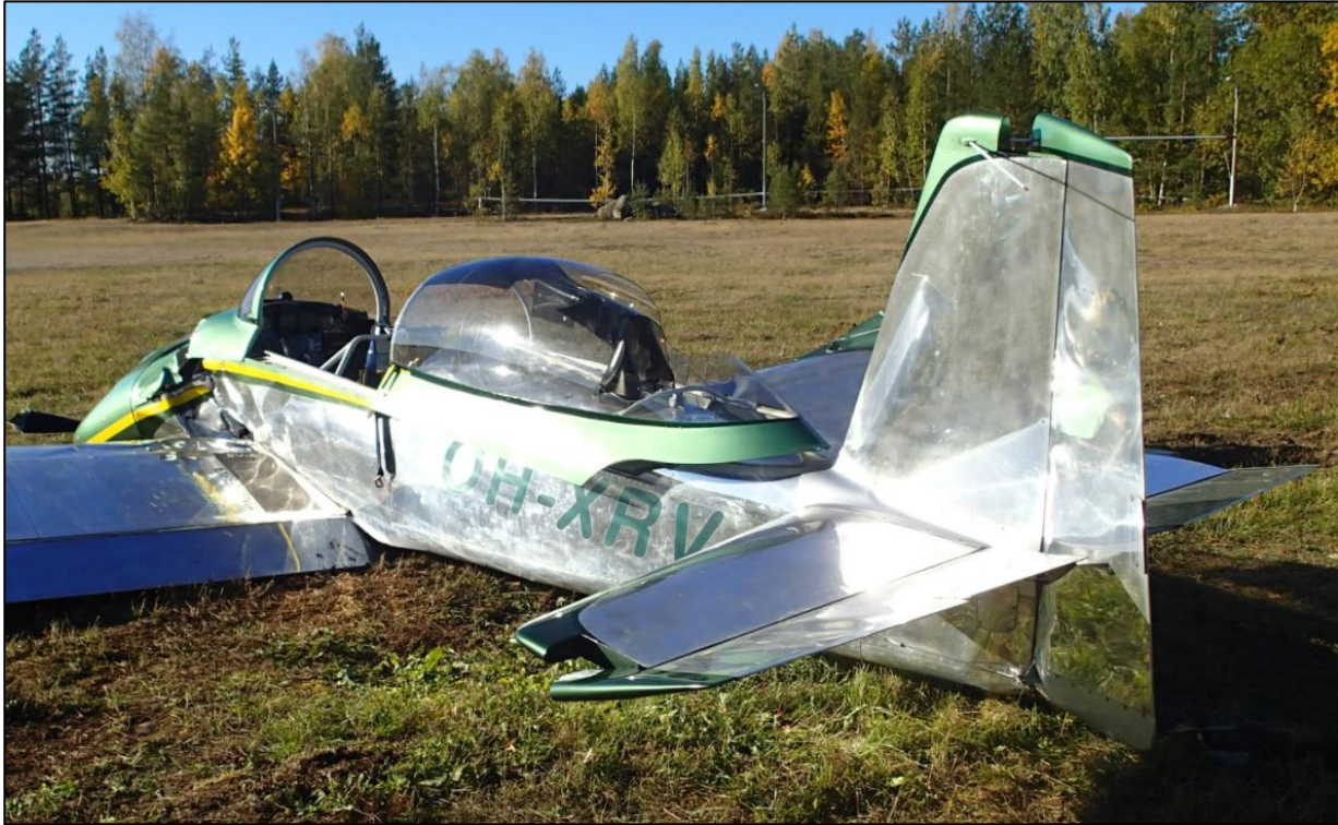
Figure 6. The side rails were distorted. An approximately 40 cm diameter hole is evident in the rear of the canopy. (Photo: SIAF)
