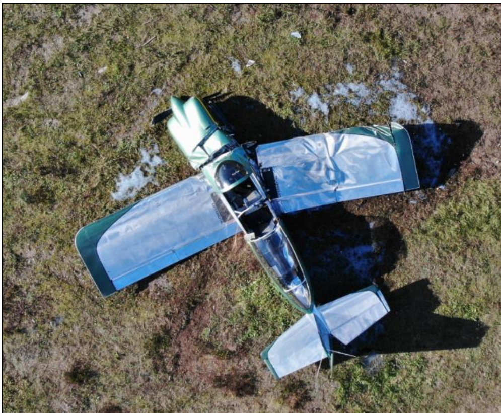
Figure 4. The airplane after the ground impact. The right wing is canted aft, and its leading edge has separated from the fuselage. (Photo: Police)
