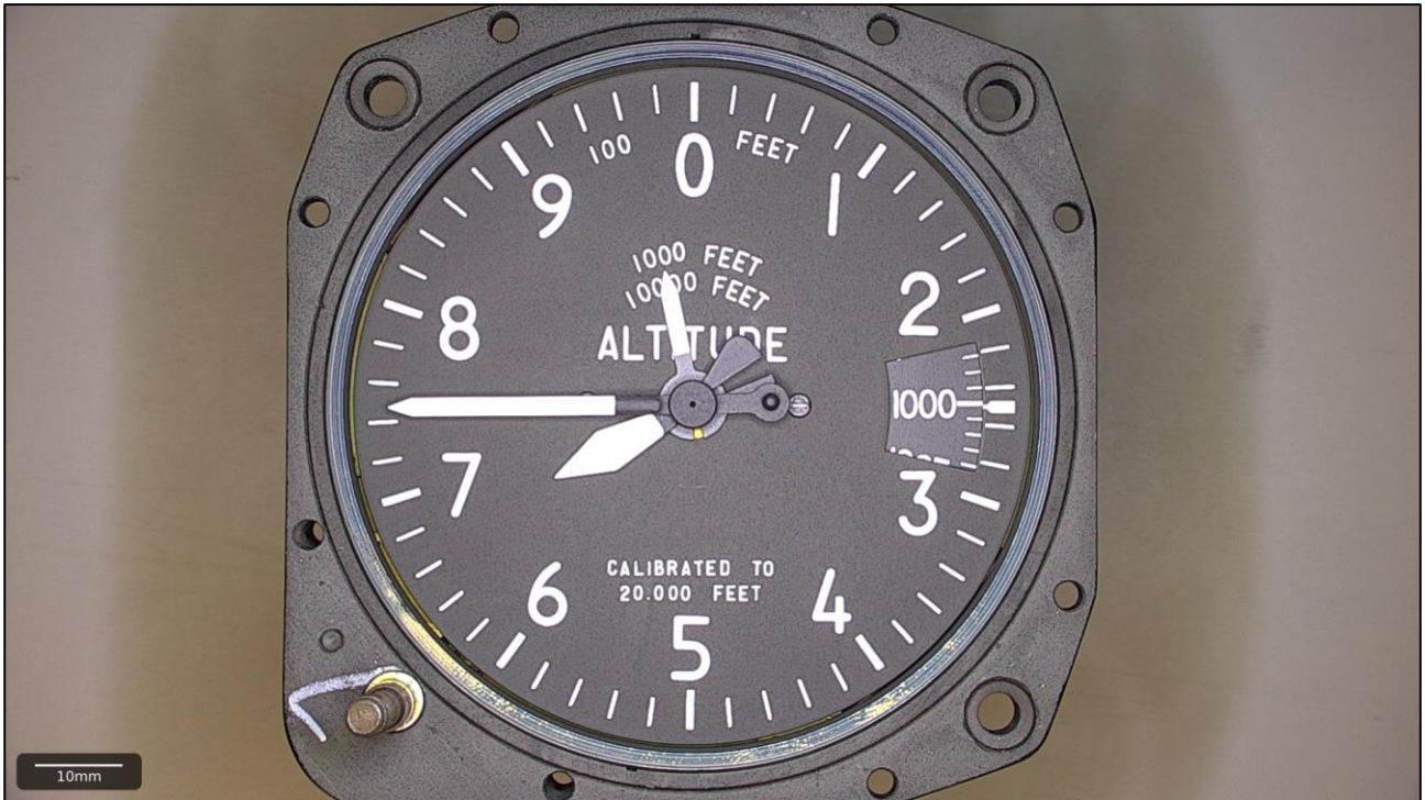
Figure 17. Altimeter indication after barometric pressure reset. (Photo: Insta ILS, usage rights: SIAF)
