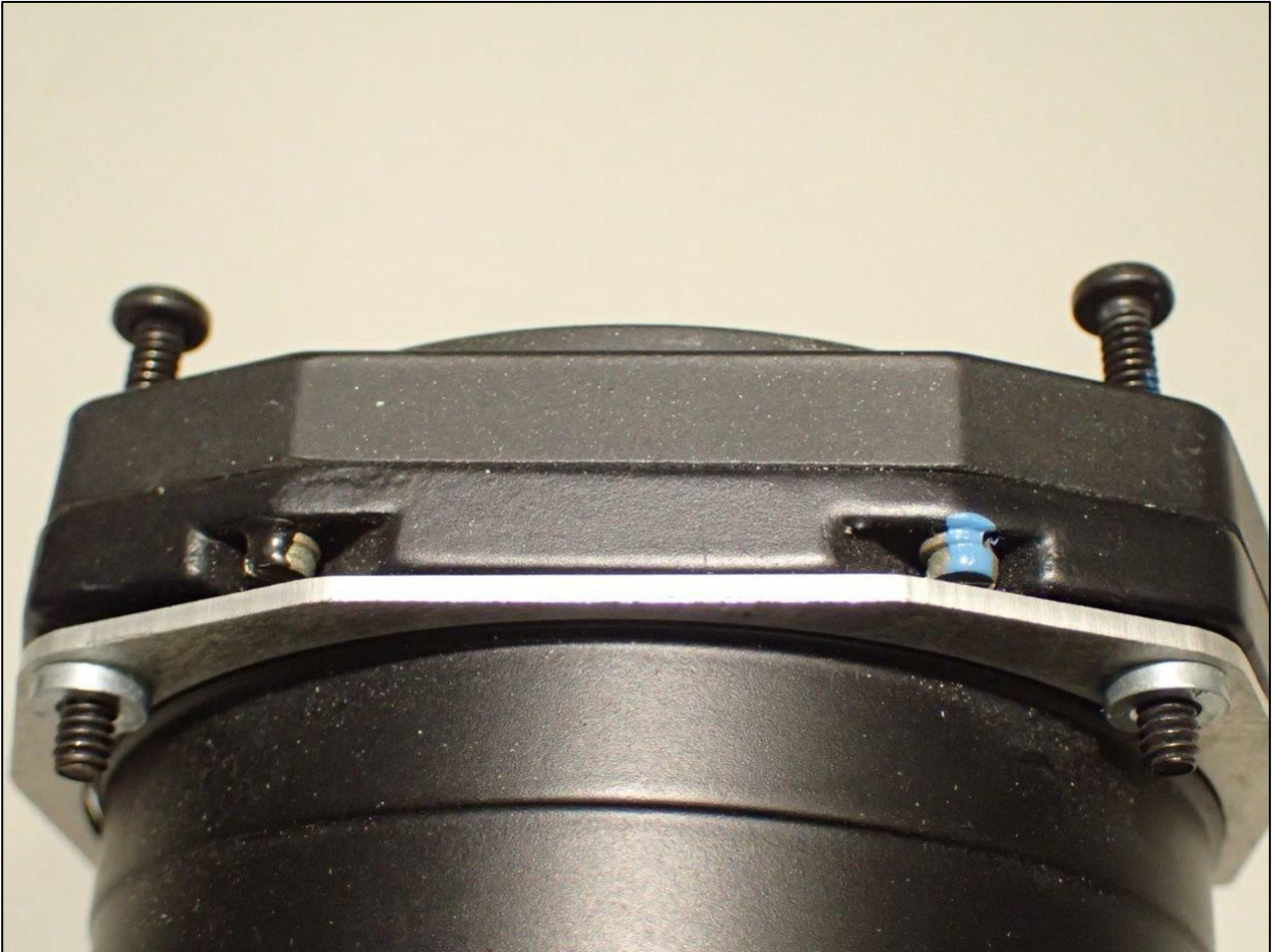
Figure 16. Altimeter case lockscrews. The left-hand and right-hand screws are sealed with black and blue paint, respectively. (Photo: Insta ILS, usage rights: SIAF)
