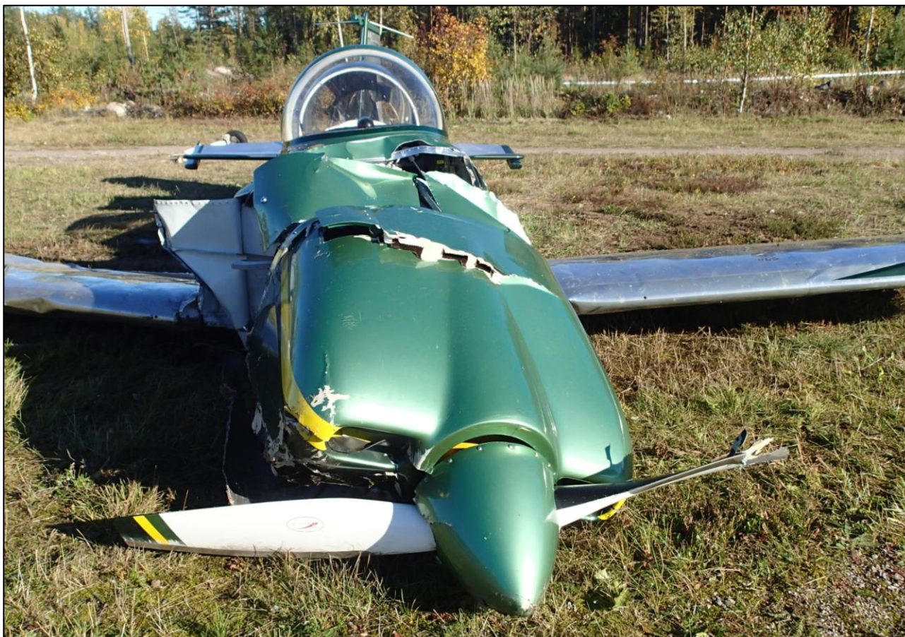
Figure 5. Fuselage damage and the partial separation and twisting of the nose section are apparent. (Photo: SIAF)
