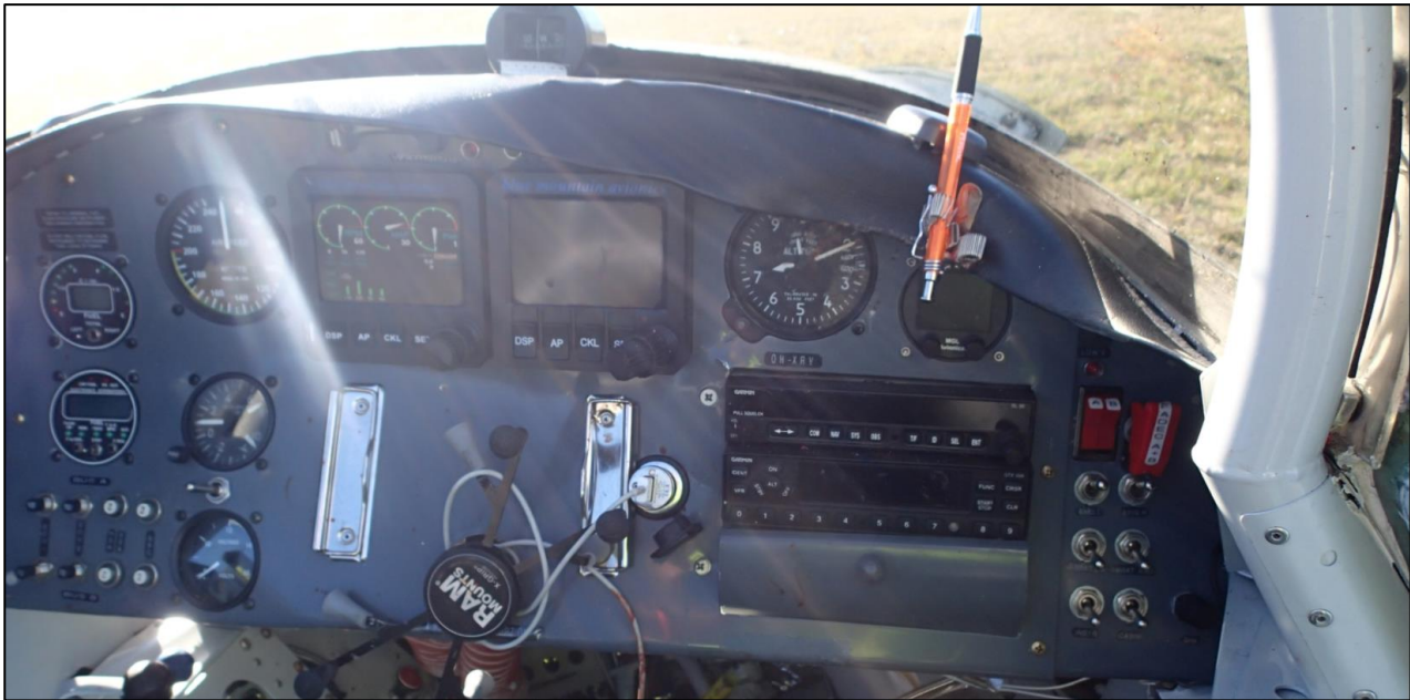
Figure 7. The instrument panel was bent at mid-point. Deformation of the glareshield is also shown. (Photo: SIAF)
