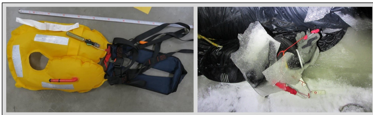
Figure 29. Photos of survival equipment. On the left, an inflatable life jacket that had been packaged or put on incorrectly, which is why it did not work as intended. On the right, an example of the attempt of a person who fell through the ice to use ice picks. (Photos by the police)
