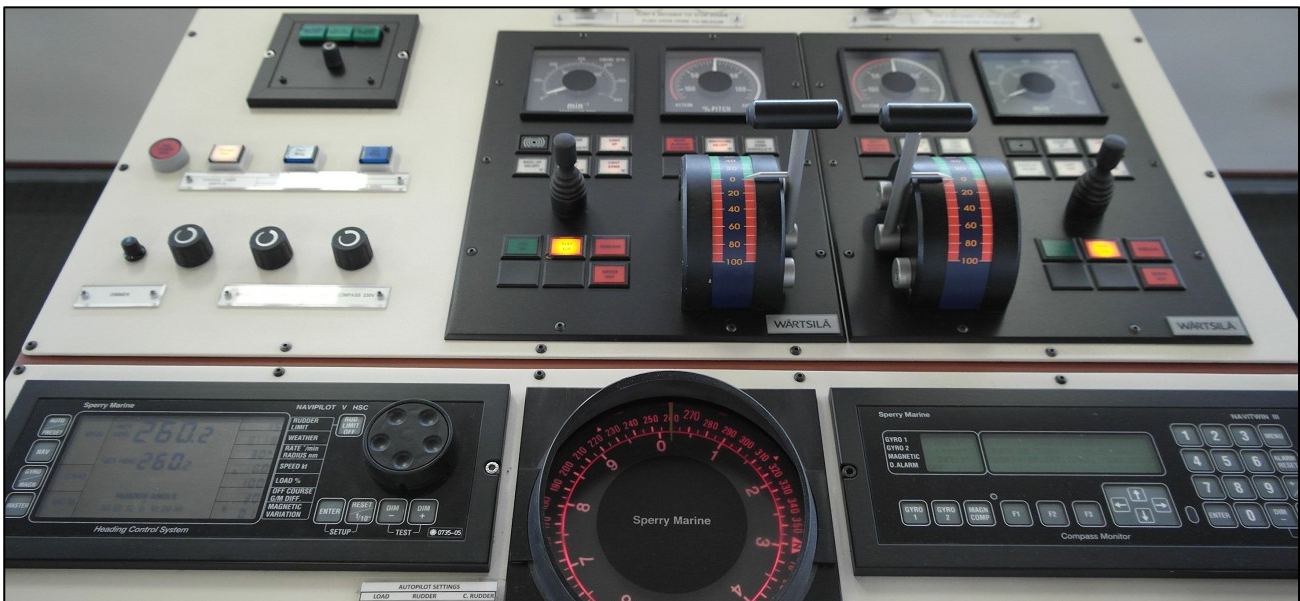
Picture 10. The image shows the control devices for the vessel's steering and machinery. (Image: SIA)
