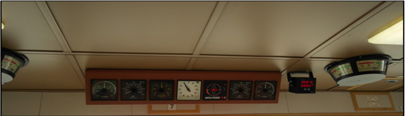
Picture 9. Ceiling console displays, a separate heading display, panoramic rudder angle displays. (Image: SIA)
