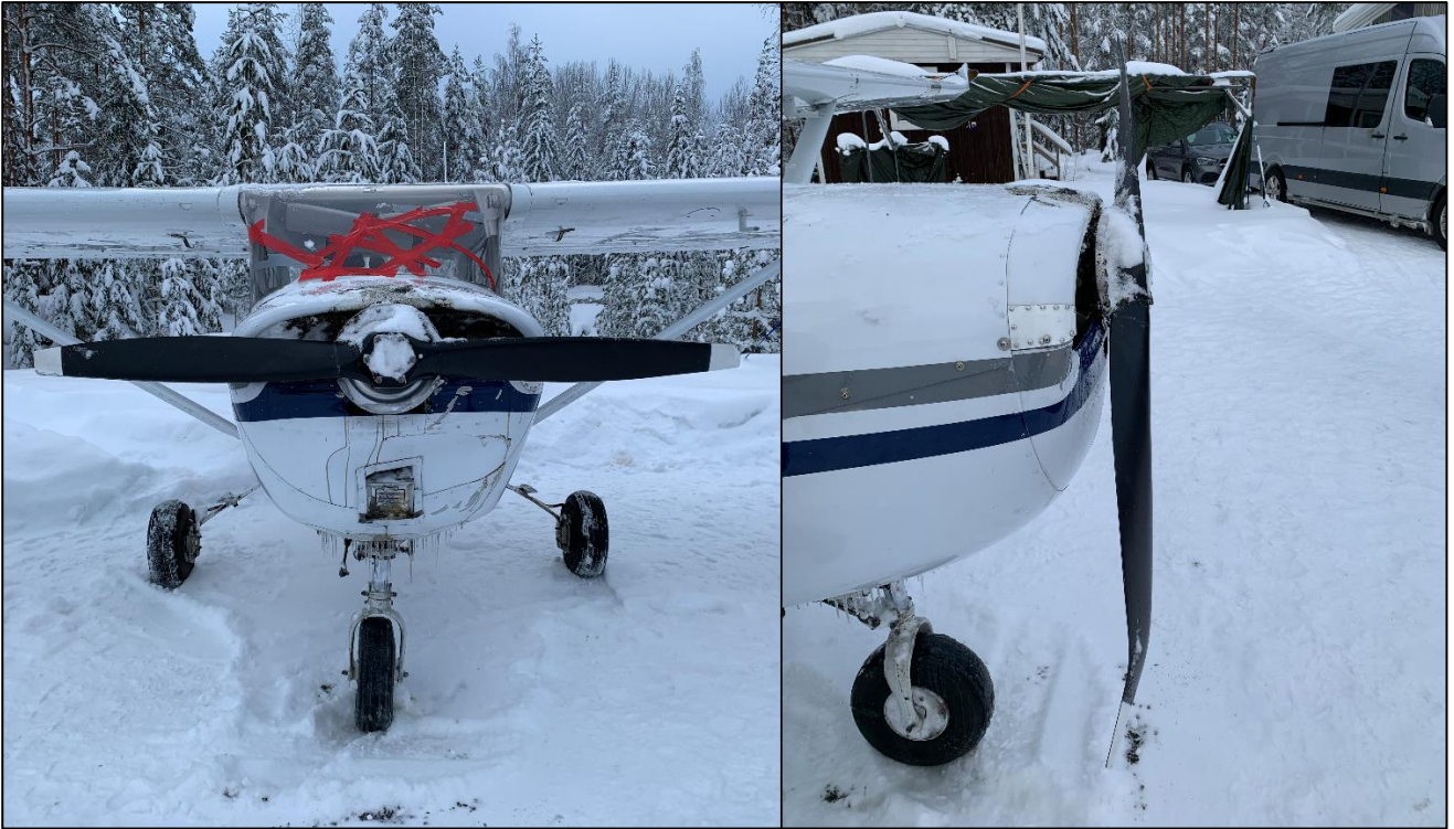
Figure 3. The windshield was cracked, and the propeller sustained damage. The red tapes were applied to the windshield after the accident. (Photos: SIAF)
