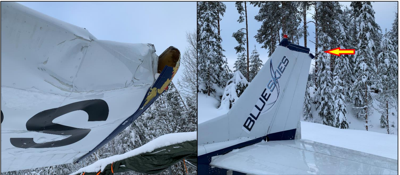
Figure 4. The left wing tip exhibited skin tear and deformation. The tip of the vertical stabilizer was damaged. (Photos: SIAF)
