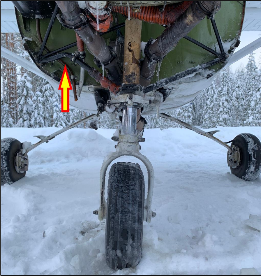
Figure 5. The nose landing gear and the engine mount (arrow) were damaged. (Photo: SIAF)
