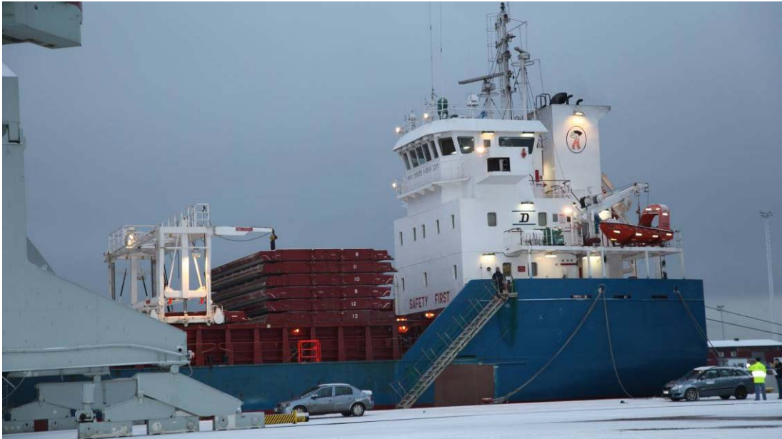
Picture 2. Hatch cover gantry crane in which the quay-side hoisting apparatus can be seen above the hatch-covers. The accident hoisting apparatus is on the SB-side.
