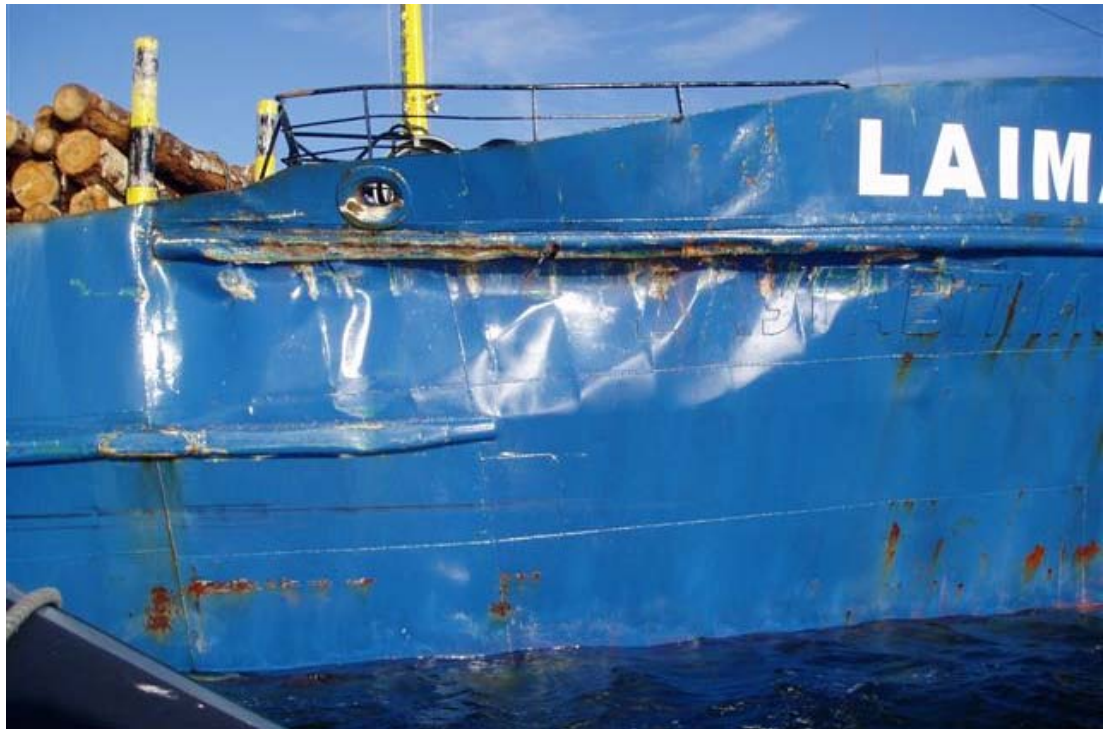
Figure 8. The damage to the LAIMA's starboard bow - external view. (Photo: Finnish Coast Guard)
