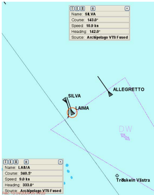
Figure 5. At 05:59:23 the vessels are approximately 0.33 miles away from one another. The LAIMA informs the SILVA that she is turning to port. This is not heard in the VTS recording; instead it can be made out that the LAIMA asks the SILVA three times to turn to port. The SILVA makes no reply and turns to starboard. The vessels turn in more or less the same direction at the same time - westward.
