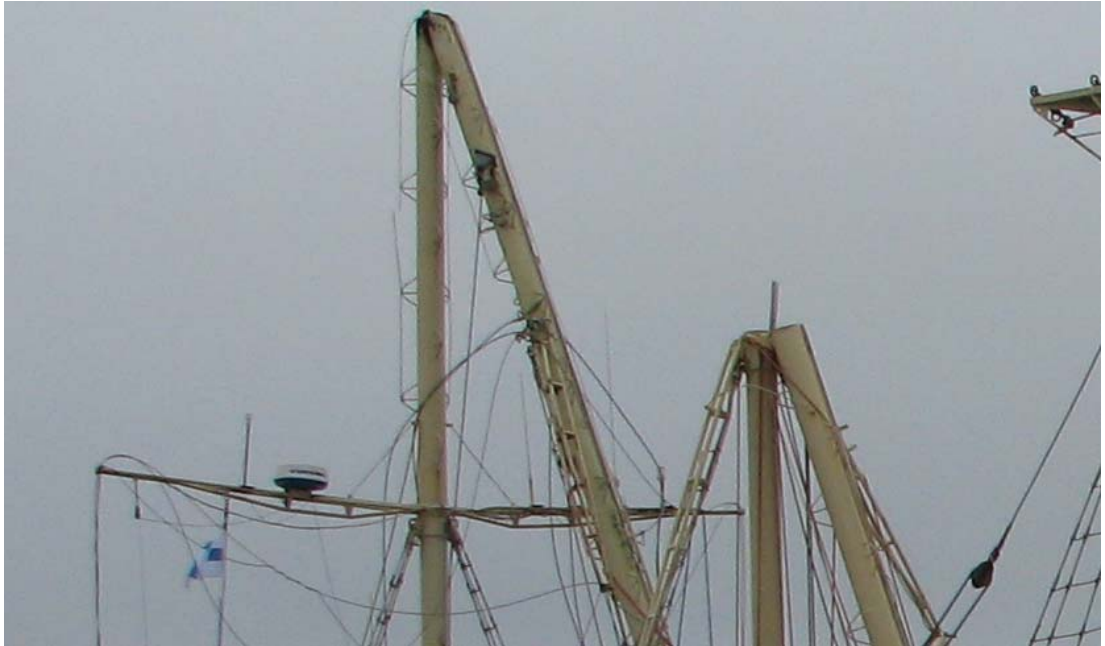
Figure 7. The bended Mizzen Mast.
