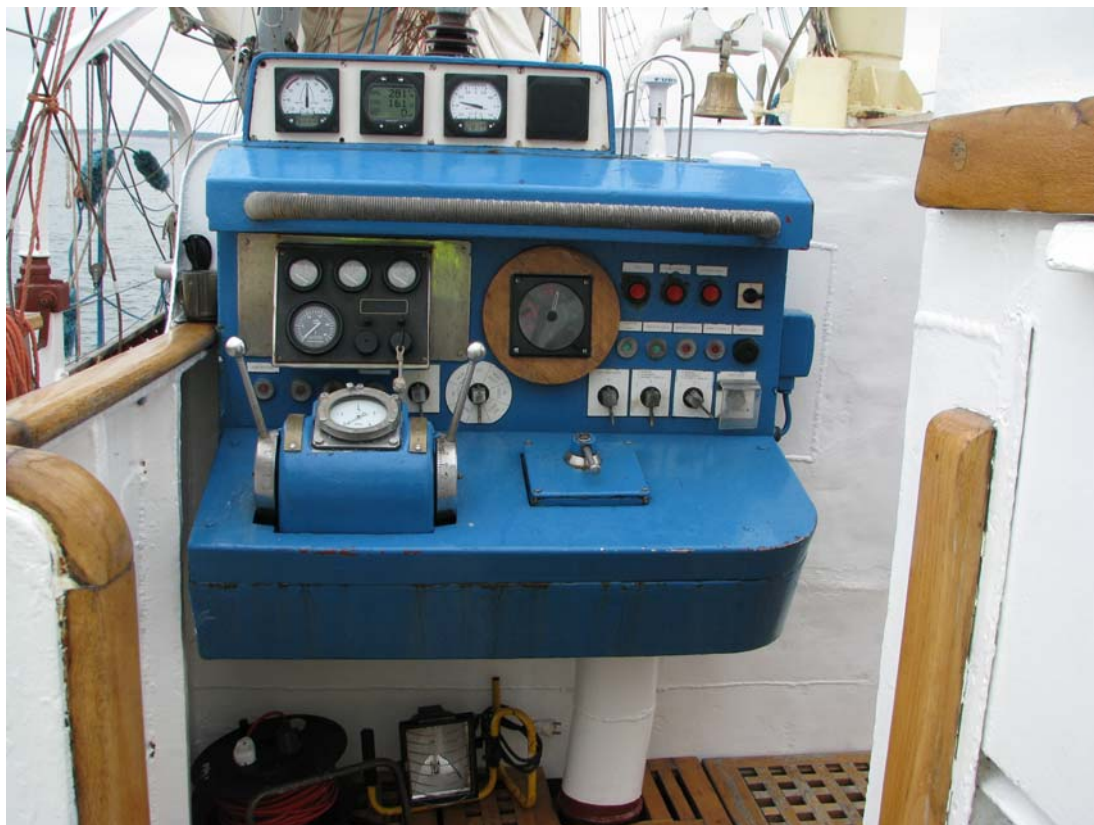
Figure 3. Manoeuvring pulpit on Port side aft. The Navigating bridge and Radio station are on the right inside the deckhouse. Engine was not in use when the accident occurred.
