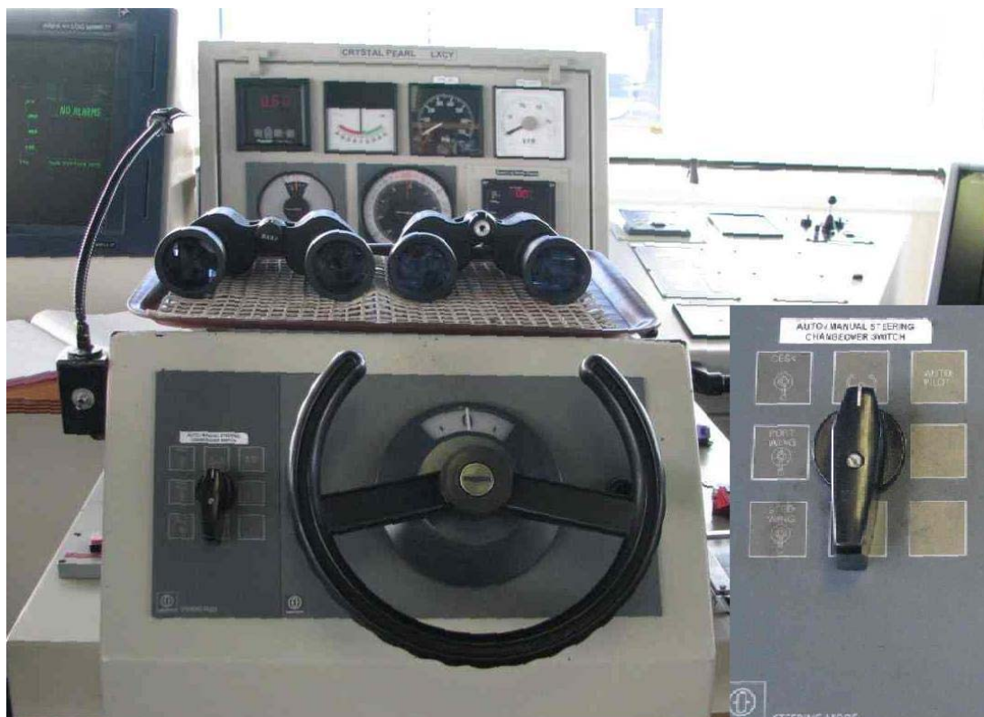
Picture 5. Steering stand for Follow-up mode in hand steering. Selector for steering post and mode enlarged on right; switch in FU hand steering position. Right top position = Autopilot selected, Left top = Desk panel NFU selected. Two lower positions on left = selections for NFU steering at the Bridge Wings.
