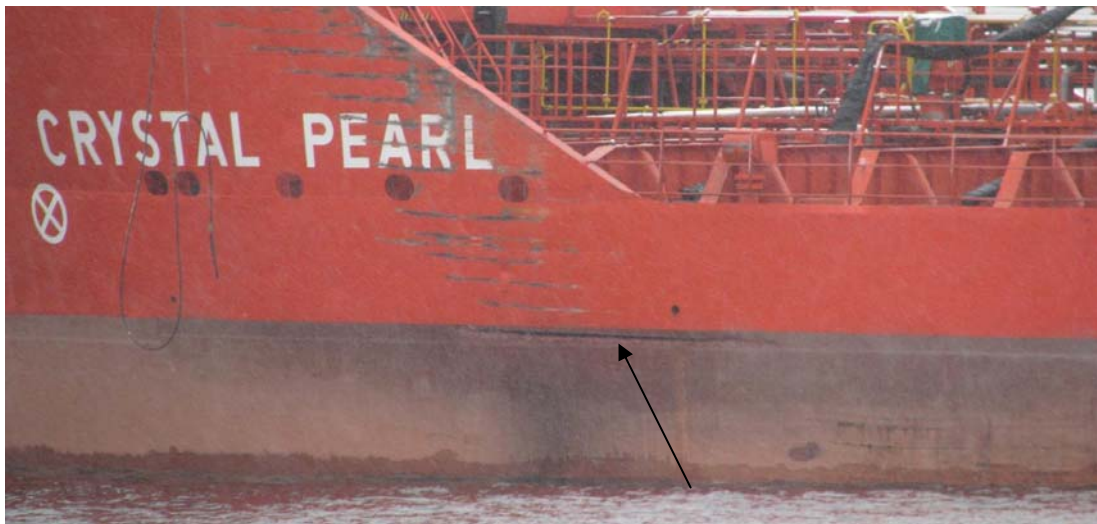
Picture 15. The arrow points the crack area on port alongside of the ship.
