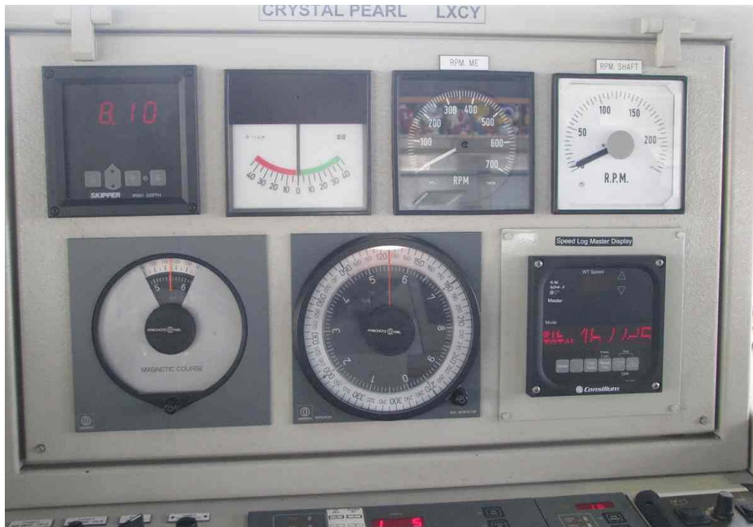
Picture 4. Displays and repeaters in the forefront console for navigation sensors, rudder angle and RPM's. On the top row from left are echo sounder, rudder angle, main engine RPM, shaft RPM. On the lower row from left; magnetic compass, gyro compass and speed log
