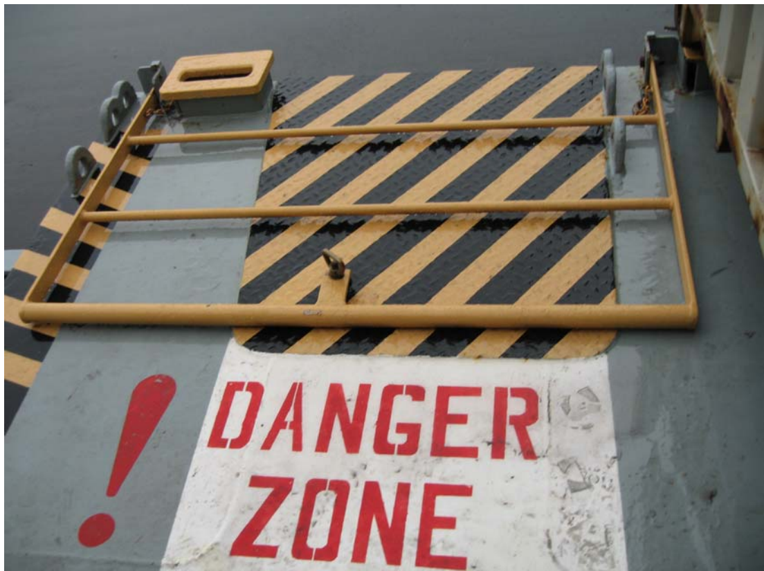
Figure 7. The safety rail and danger zone markings on the starboard side.
