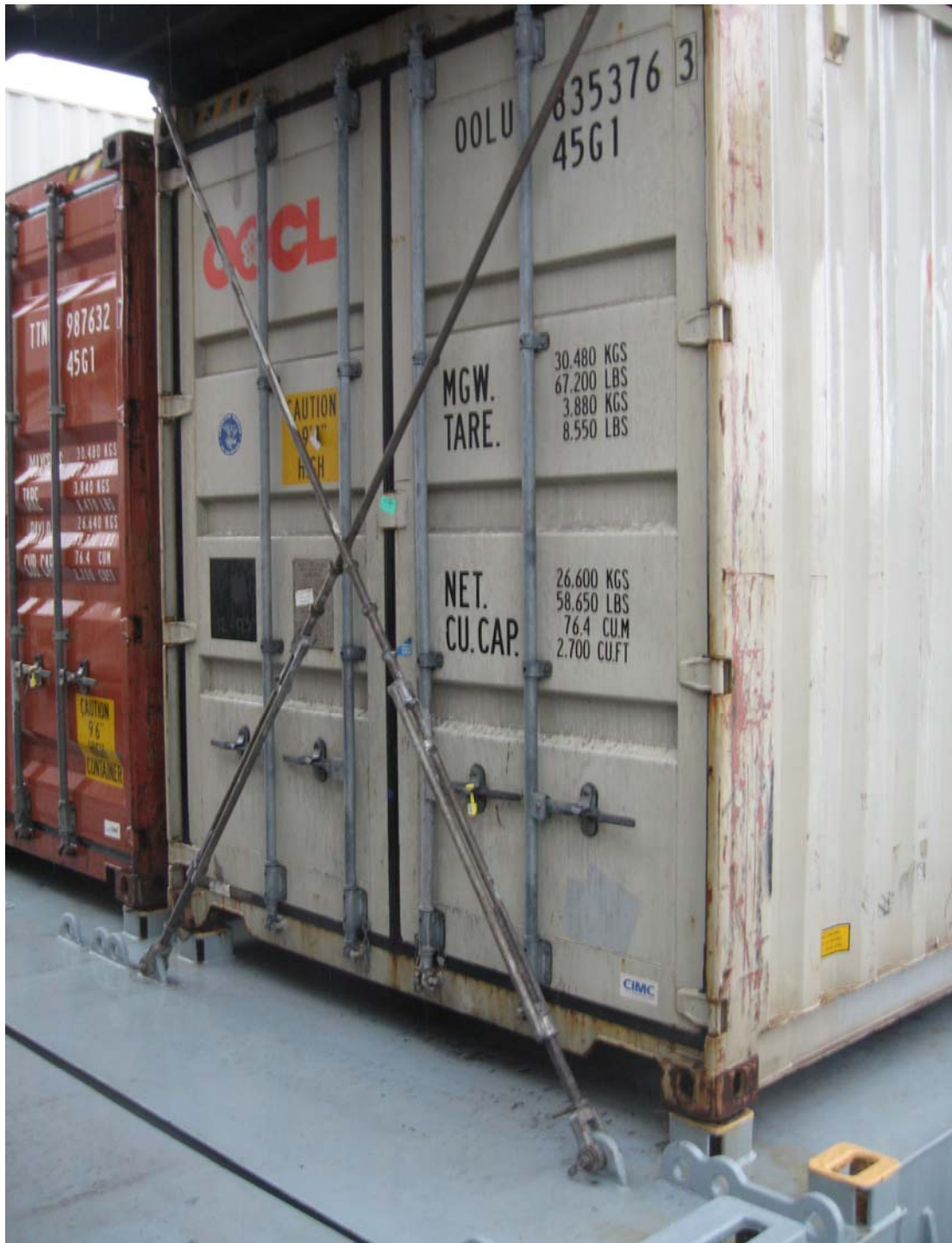
Figure 2 A container lashed to the deck.
