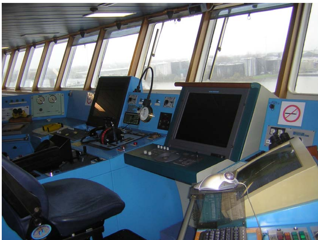
Figure 6. Wheelhouse on BIRKA EXPORTER. The closest chair was the conning position prior the collision.
