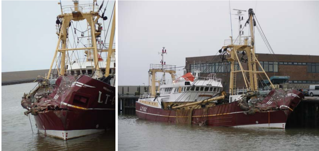
Figure 16a and b Damages to HENDRIK SENIOR above waterline.
