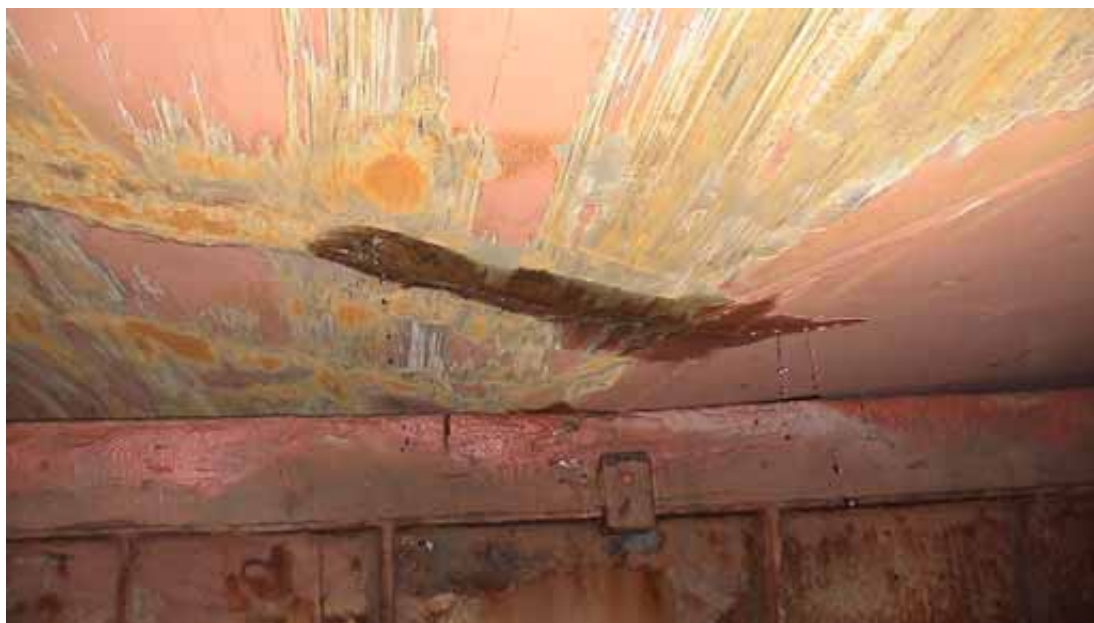
Figure 7. Minor crack in ship's bottom ballast tank.
