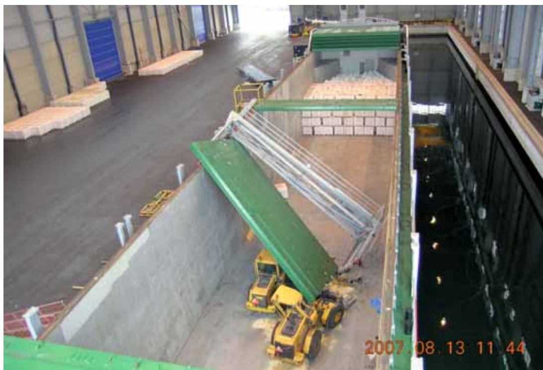
Figure 2. The hatch cover and the crushed tractor in the cargo hold.
