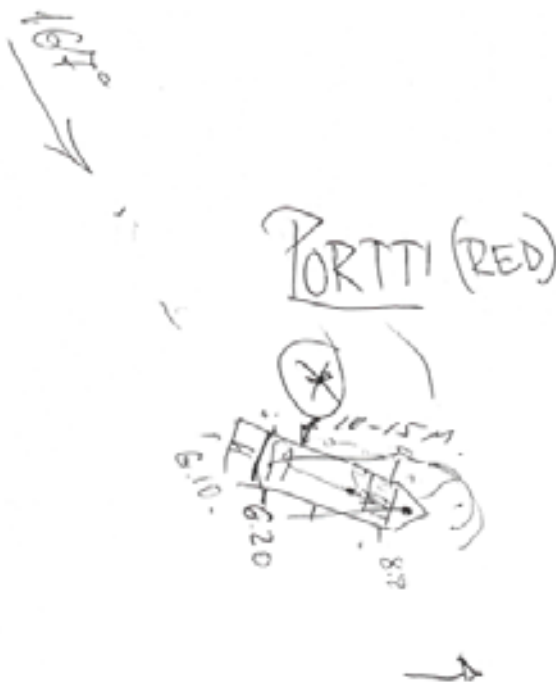
Figure 7. A drawing made by the chief officer on the location of the grounding. The drawing describes how the vessel turned after running aground. When grounding, the course of the vessel was 120°.
