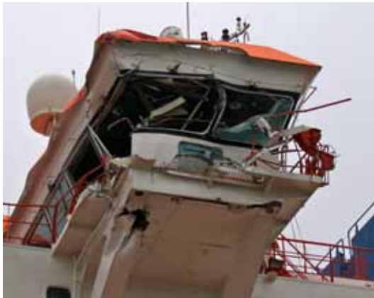
Figures 16 and 17. The portside wing of the vessel (Figure 16, left). The portside steering equipment console (Figure 17, right). (the pictures on behalf of BSU)
