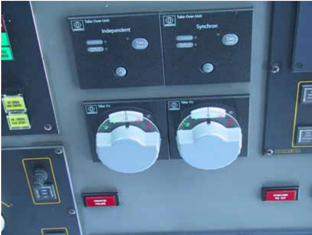
Figure 8. The Follow Up control of the rudders on the bridge wings.
