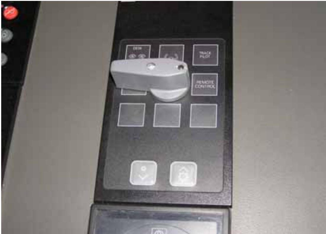
Figure 7. Selection of rudder control point in the console of the helmsman.
