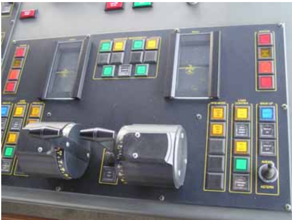
Figure 5. The control levers for the main propellers. The master used these.
