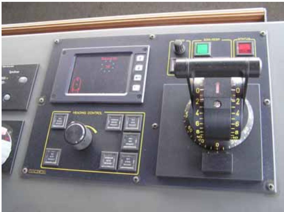
Figure 9. The KaMeWa Joystick, efficient for harbour manoeuvring.
