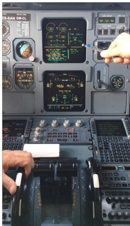
Figure 42 Actuation of the pitch trim wheel
