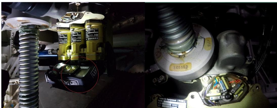
Figure 43 Camera recording the PTA micro-switch movement
