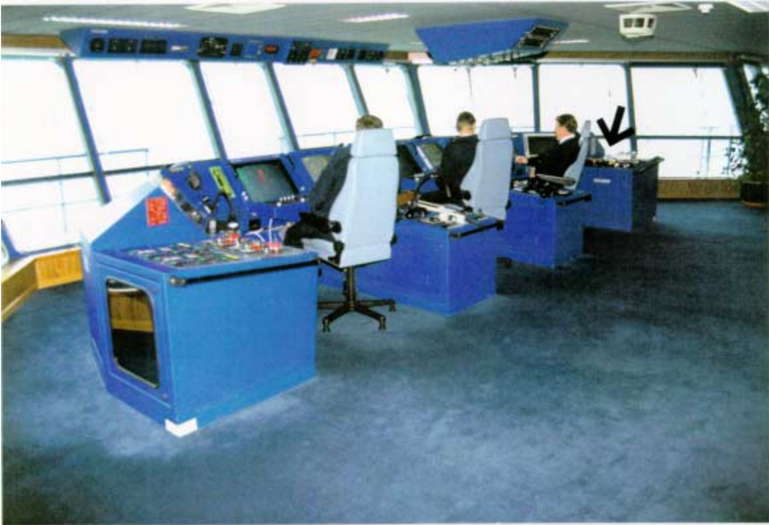
The navigation desk on the bridge of the M/S SILJA EUROPA. The arrow indicates the location of the BY-PASS switch.
