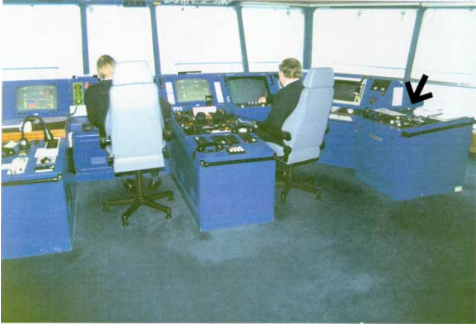
Close-up of the navigation desk. At the time of the accident, the pilot sat on the left and the officer of the watch sat on the right. The arrow indicates the location of the BY-PASS switch.
