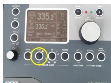
Fig. 6. Steering control system unit ALPHASEAPILOT in standby (STBY) mode
