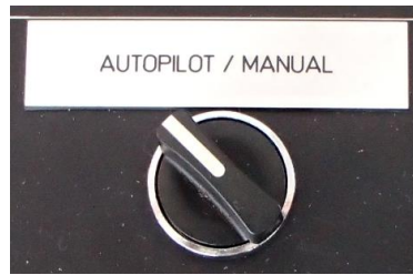
Fig. 7. Steering mode selector lever in position AUTOPILOT
