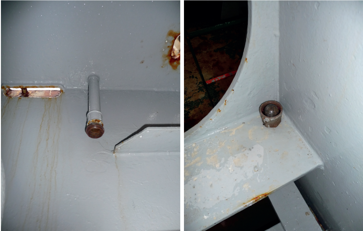
Figure 11: Left: drainage pipe without cap; right: watertight sealing cap with non-return valve. (Photo's: Dutch Safety Board)
