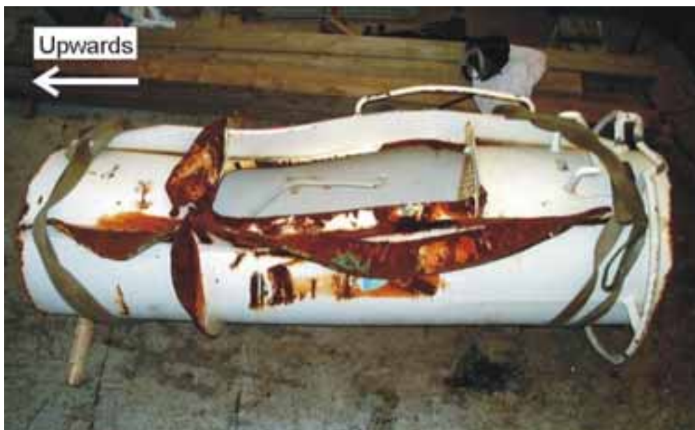
Figure 27. Position of the impact on Tröskeln Västra. In the middle is the door opening.
