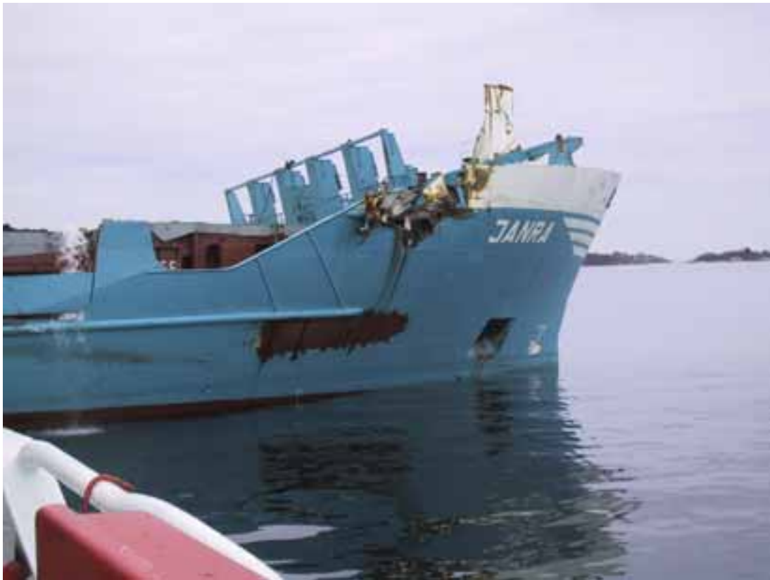
Figure 24. The two areas of damage on the bow of the JANRA. The photograph has been taken after the ship had been turned. (The lower hole had been temporarily repaired under water.)
