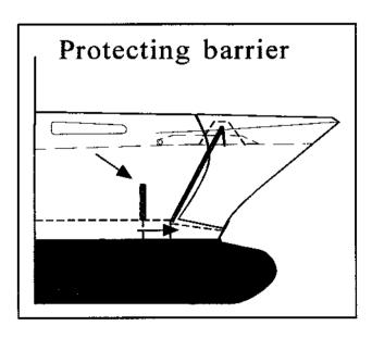
M/S Estonia had a garage built on the visor to accommodate the upper part of the ramp. The ramp was moved forward and therefore did not fulfill the rules as an extension of the collision bulkhead. The arrangement could have complied with the rules of SOLAS if an additional barrier had been arranged.
