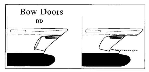
A bow visor forms the bow on a ship. The visor is normally hinged on the forecastle deck and is opened upwards by hydraulic cylinders. The visor's supporting structures in the hull doesn't prevent the visor from opening. Only the locking devices have that function. The space between the visor and the ramp is sealed to the sea along the visors contouring frame. Depending on the geometry of that frame and the elasticity of the visor the frame may absorb some of the forces acting on the visor.
