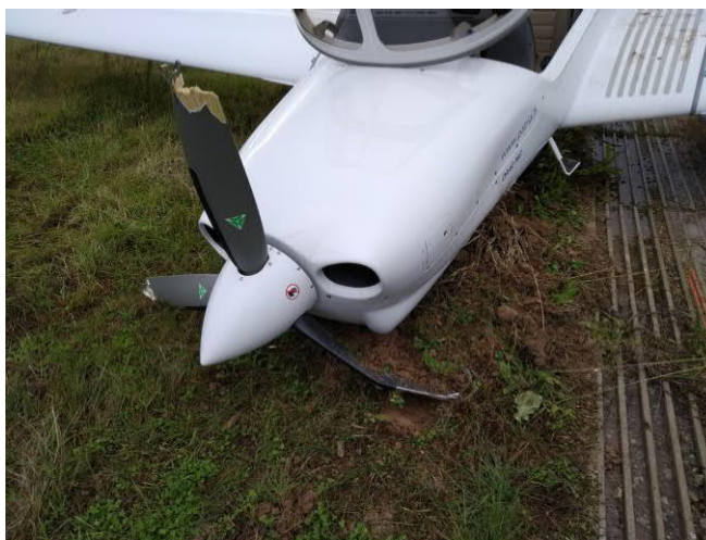
Figure 4. Damage to the propeller blades
