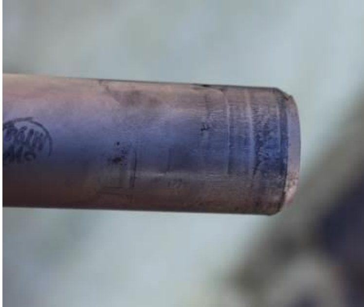
Kuva 4. The aft end of the right main landing gear forward pivot pin, photographed after the accident. This end is attached to the landing gear trunnion. Photo: Lapin Tilauslento Oy
