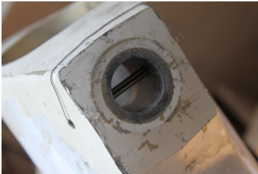
Kuva 5. The securing pin of the right main landing gear forward pivot pin in place after the accident. Photo: Lapin Tilauslento Oy
