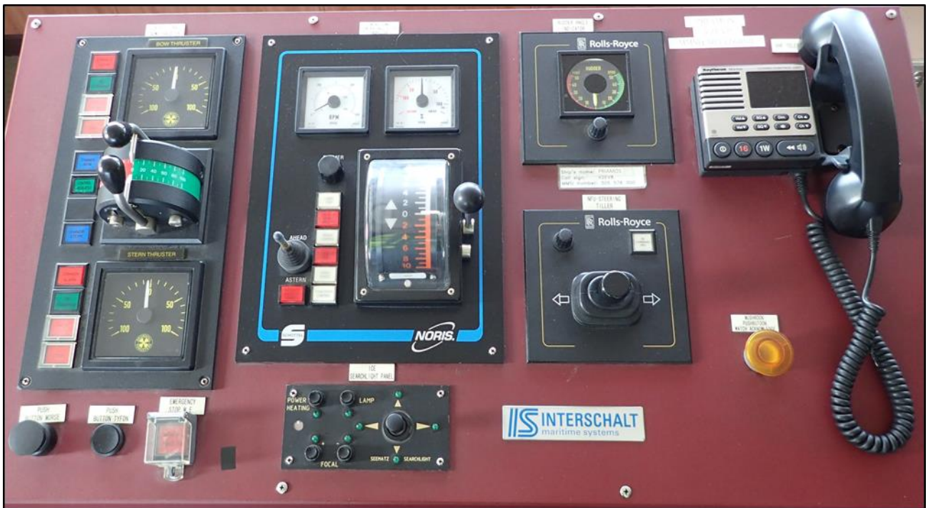
Picture 13. A close-up of the steering console in the left wing from which the pilot steered the vessel. On the bottom left is the display of the stern thruster and control lever, correspondingly, the lever and display of the bow thruster are at the top. In the centre, there are the control levers of the main engine and the propeller, and above them the displays for the rotation speed (main engine and propeller) on the left and the propeller pitch displays on the right. On the right, there is the rudder control and display, as well as a phone. (Photo: SIA)
