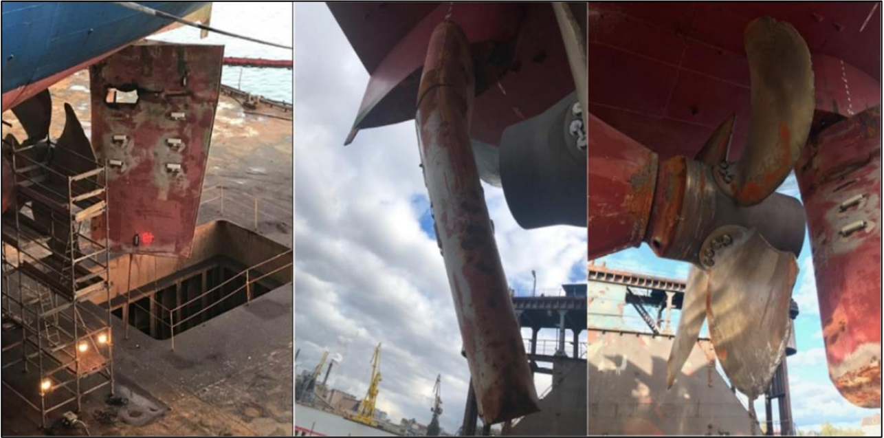
Picture 4. The vessel's damaged rudder on the left, the bent rudder stock in the middle, and the damaged propeller on the right. (Photos: Leonhardt & Blumberg, Shipmanagement GmbH & Co. KG)
