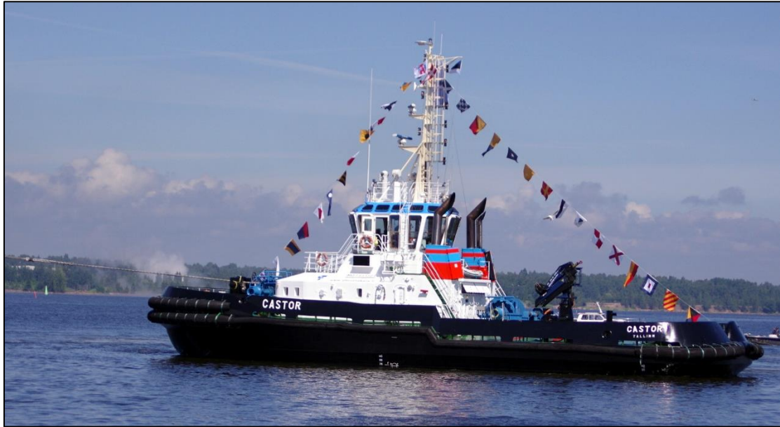
Picture 7. Tugboat Castor. Castor's length is 34.5 m, width 12.10 m, draught 4.5 m and SBP 65 tons. (Photo: Alfons Håkans AS)
