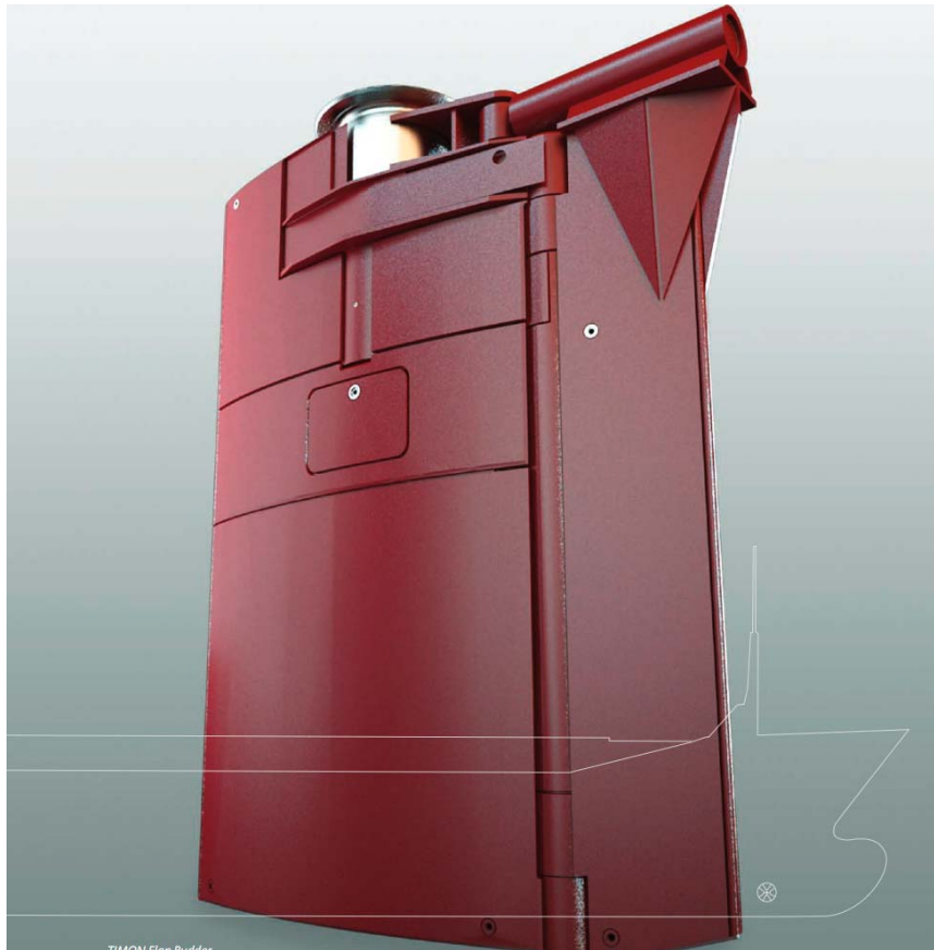
Figure 3. The TIMON rudder (Photo: van der Velden Marine Systems B.V)
