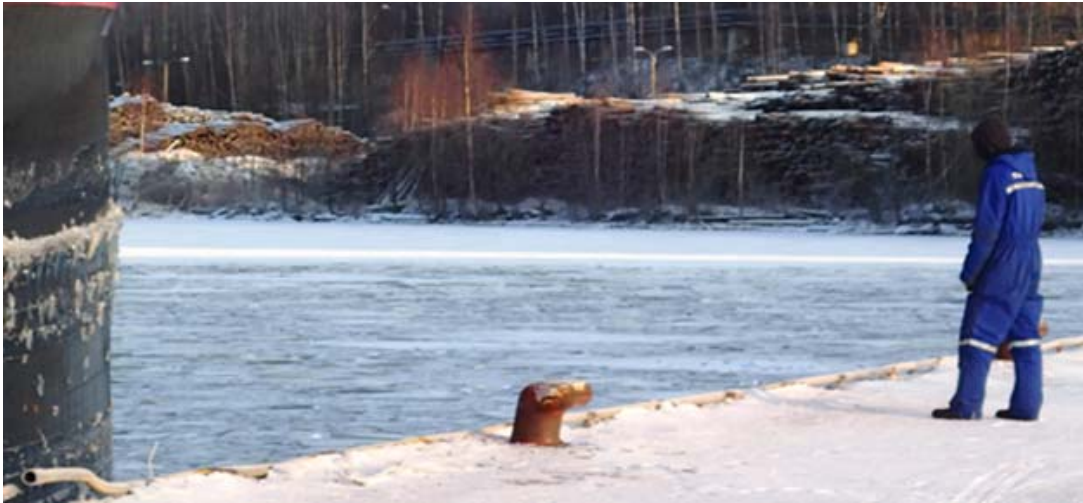
Figure 13. Quay transfer of a cargo vessel in the Port of Vuoksi 14.1.2014. The seaman waiting for the bowline does not have safety equipment required in port and necessary for the safe execution of the task. The vessel and person in the photo are not related to the accident. (photo: the SIAF)
