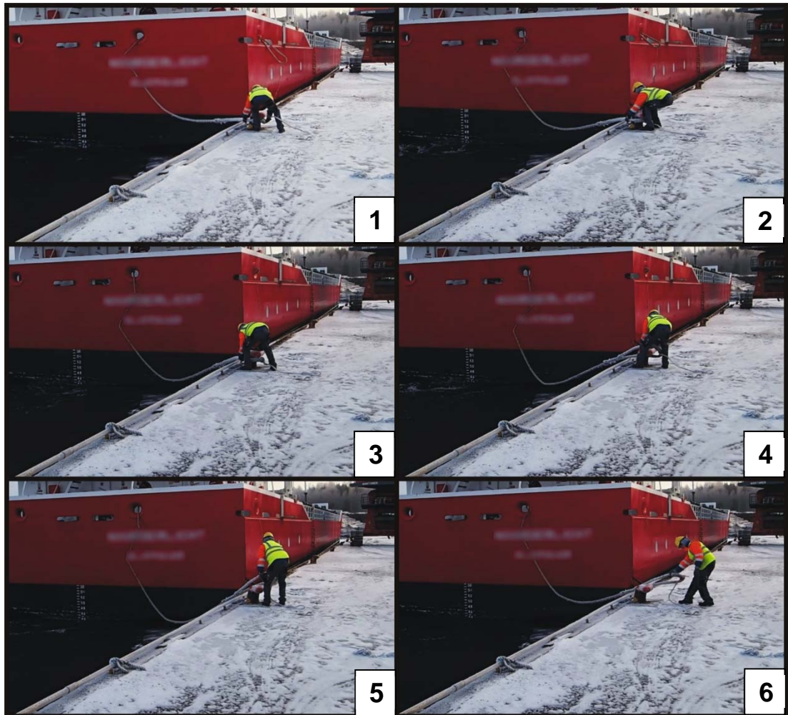
Figure 8. Series of photos portraying the actions of a line handler when letting go of a vessel similar to the accident vessel as to its size at berth number 2 in the Port of Vuoksi in winter conditions. The line handler shown in the photo had been ordered from a subcontractor, and he was not wearing a lifejacket. Photo taken on 14.1.2014. (Photos: the SIAF)
