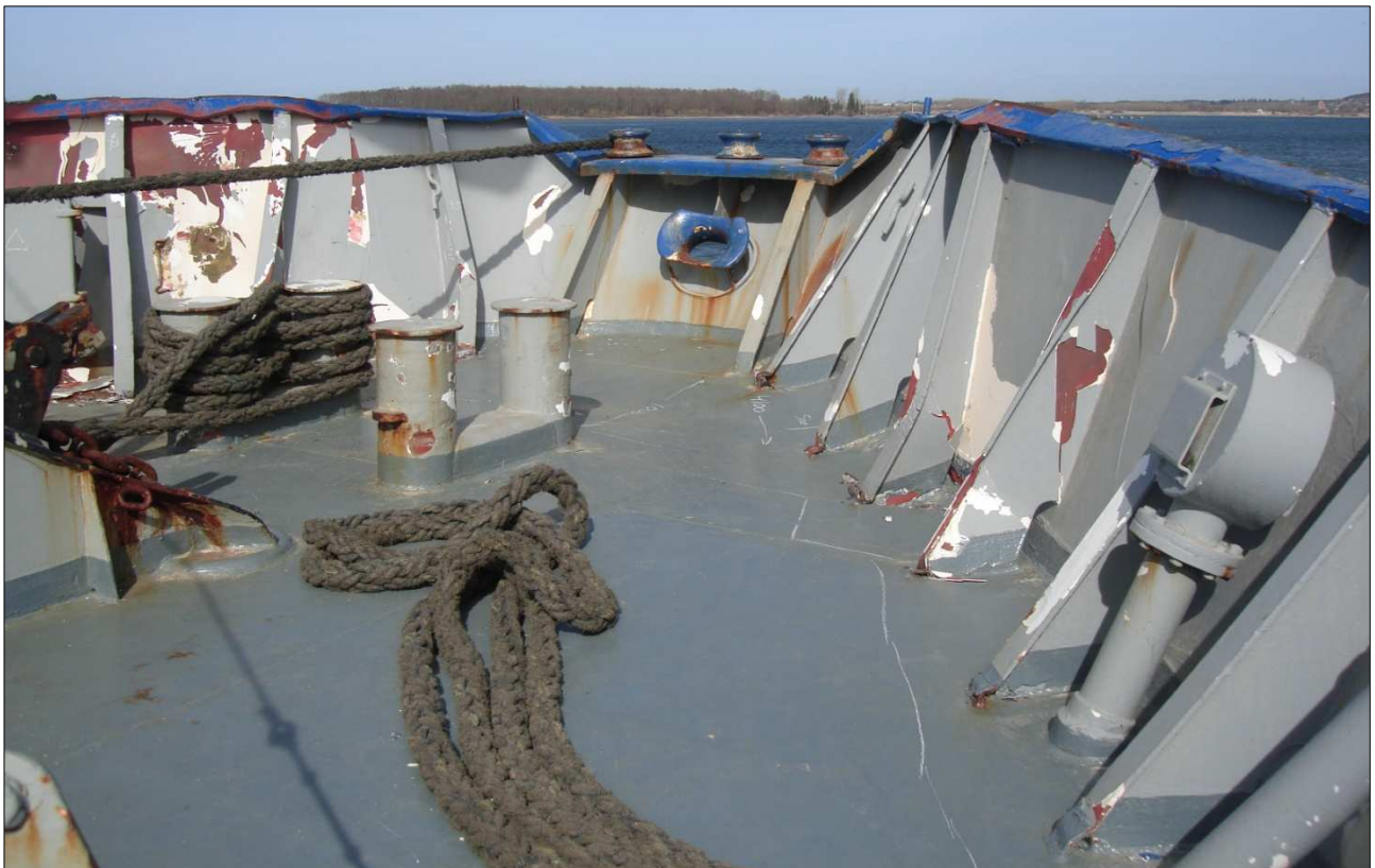
Figure 12: Damage to RAMONA after collision with the Railway Bridge Source: DMAIB
