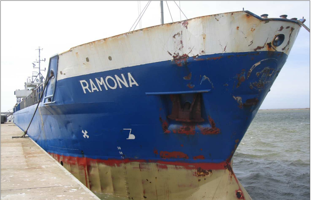
Figure 11: Damage to RAMONA after collision with the Railway Bridge Source: DMAIB
