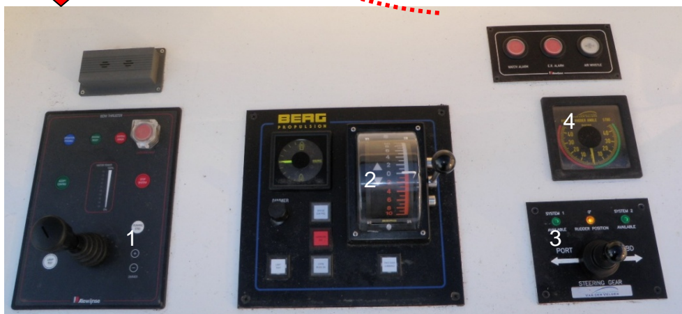
Figure 4. Bridge wing equipment: 1. Bow thruster control, 2. Controllable pitch propeller, 3. Rudder "Tiller", 4. Rudder angle indicator, 5. Sister (repeater) indicator of gyro compass (the upper figure).
