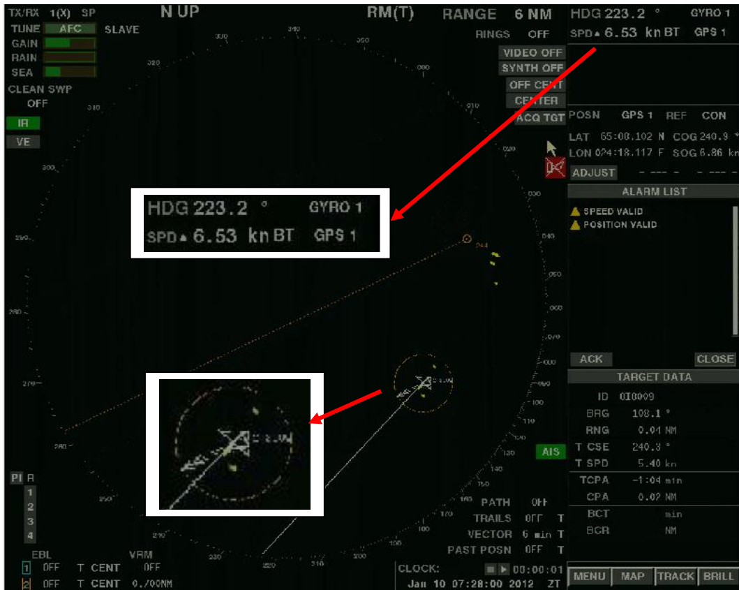
Figure 3. At 7:28:00 the Master changes the course to heading 180° upon the Pilot's request.
