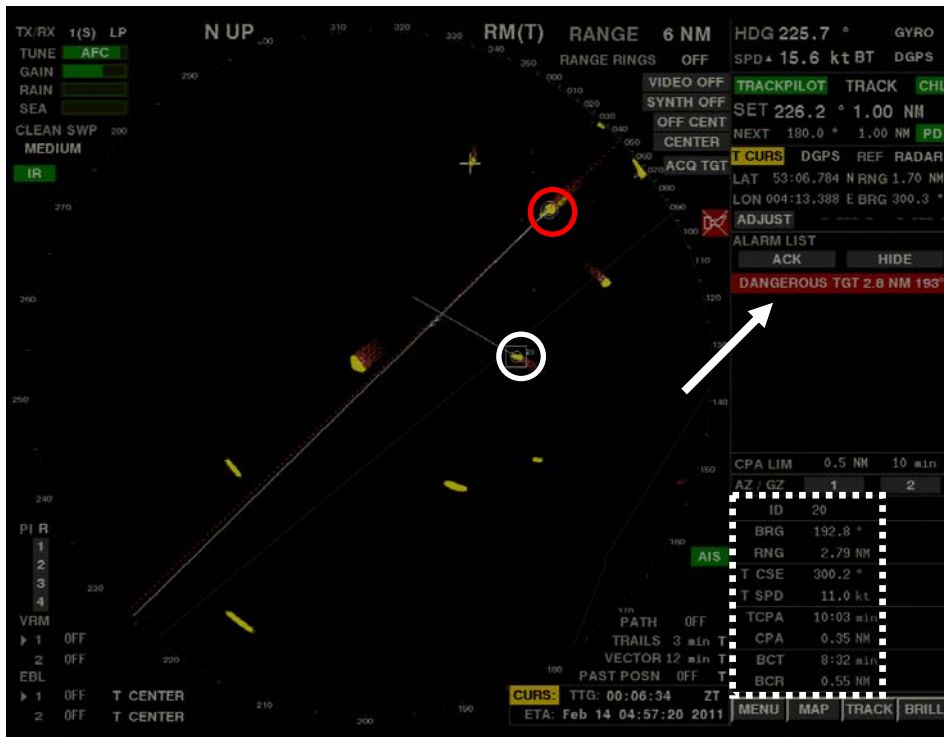
Figure 8. At 3:50:50. Time to the collision is circa 10 min. Dangerous target alarm was activated (white arrow). CPA 0.35 NM and TCPA 10.03 min.
