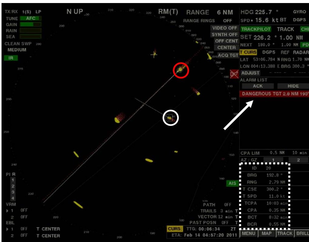
Figure 5. At 3:50:47. Dangerous target alarm is activated on BIRKA TRANSPORTER's radar (white arrow). Target limits were set at CPA 0.5 NM and TCPA 10 min. CPA 0.35 NM and TCPA 10.03 minutes. Time to the collision is circa 10 minutes. The rectangle shown in white dash lines indicates WILLEMPJE HOEKSTRA's ARPA data.
