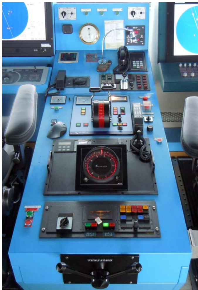
Figure 5. The helmsman's position is at the end of the main console.
