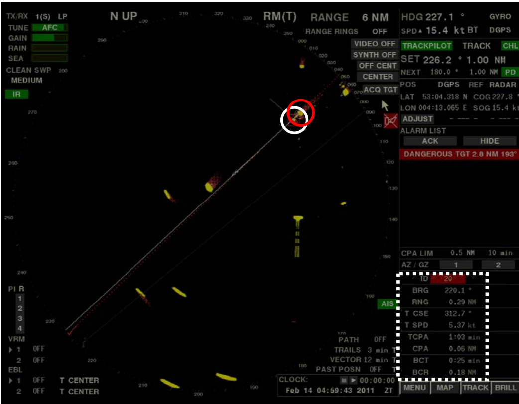
Figure 6. At 3:59:43. BIRKA TRANSPORTER's speed starts to decrease. The white circle represents WILLEMPJE HOEKSTRA, the red circle BIRKA TRANSPORTER, and the rectangle in white dash lines is the ARPA data. Time to the collision is circa 1 minute. CPA 0.06 NM, TCPA 1.03 min.
