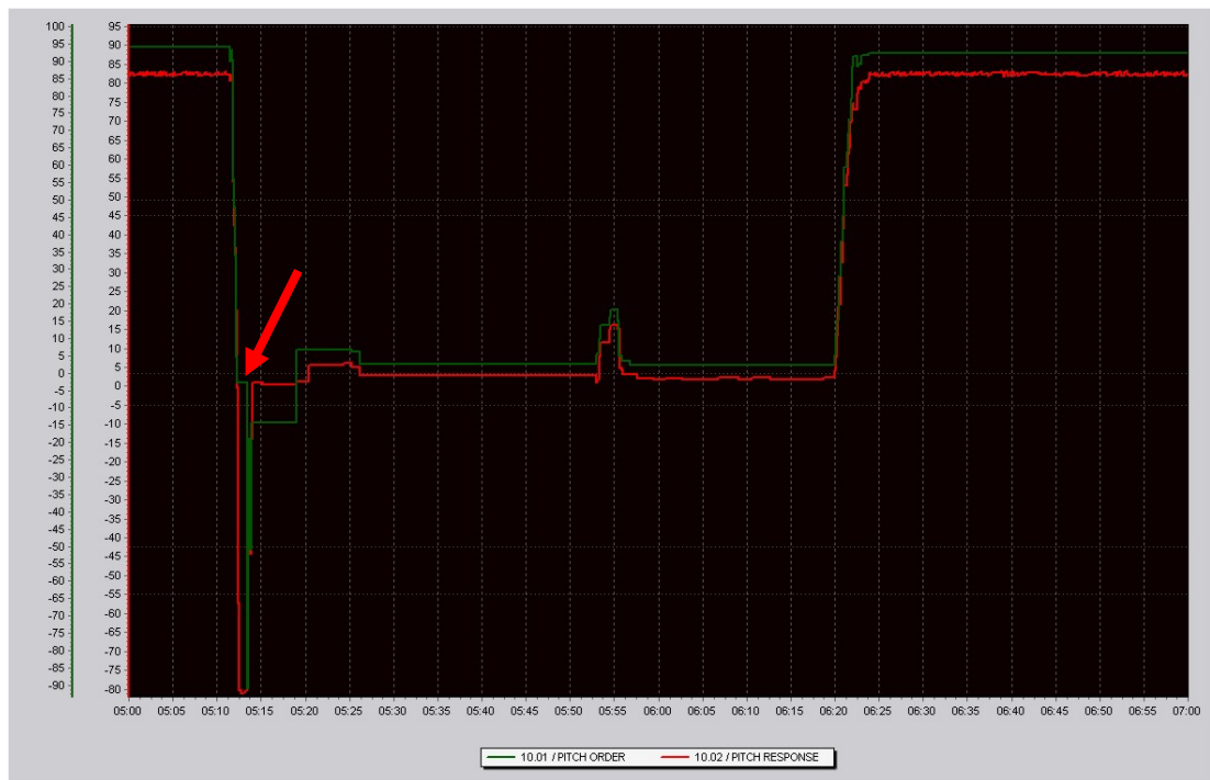
Figure 8. The pitch log from BIRKA TRANSPORTER. Pitch order is shown in green and pitch response in red. The time is approximately 12 minutes ahead of the S-VDR time.
