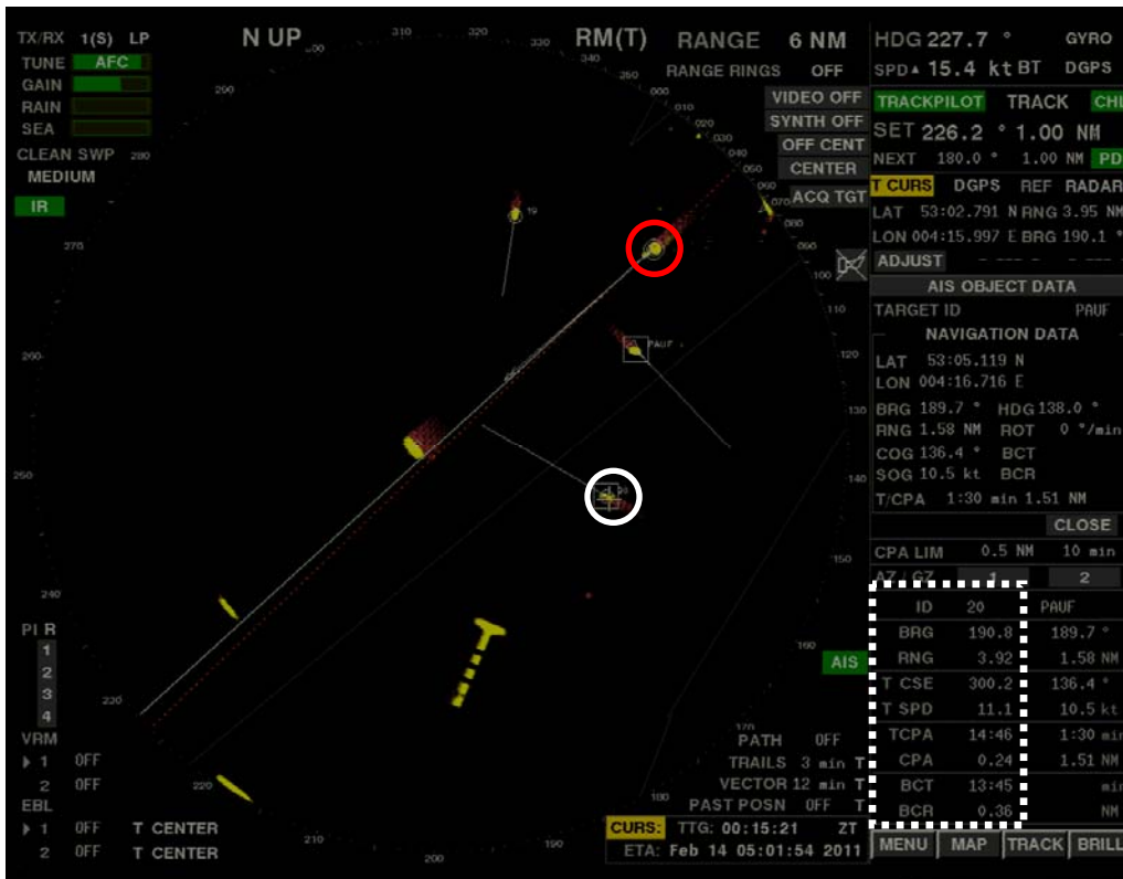
Figure 4. At 3:46:34. WILLEMPJE HOEKSTRA's (white circle) ARPA data (rectangle in white dash line) is activated on BIRKA TRANSPORTER's (red circle) radar. Time to the collision is circa 14 minutes. CPA is 0.24 miles and TCPA 14.46 minutes.
