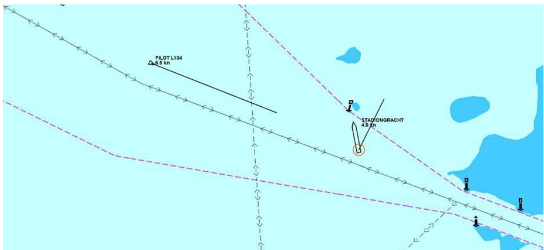
Figure 8. At 00:12:41. The VTS-operator tells to the pilot cutter that the SG has started turning via port. SG 029° / 4.0 knots.
