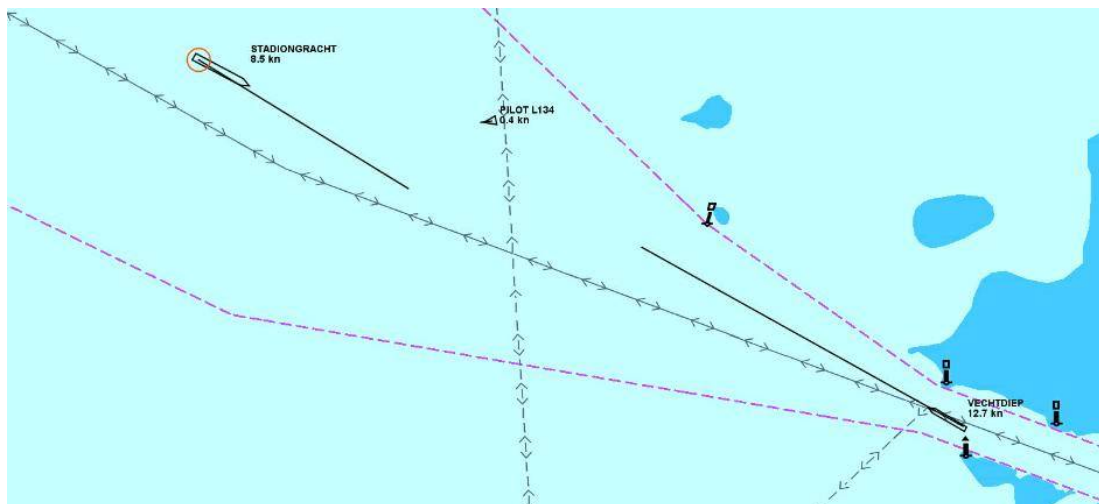
Figure 2. At 00:03:11. The cutter has stopped, VD is coming to the lateral mark RR 15. SG 120° / 8.5 knots.
