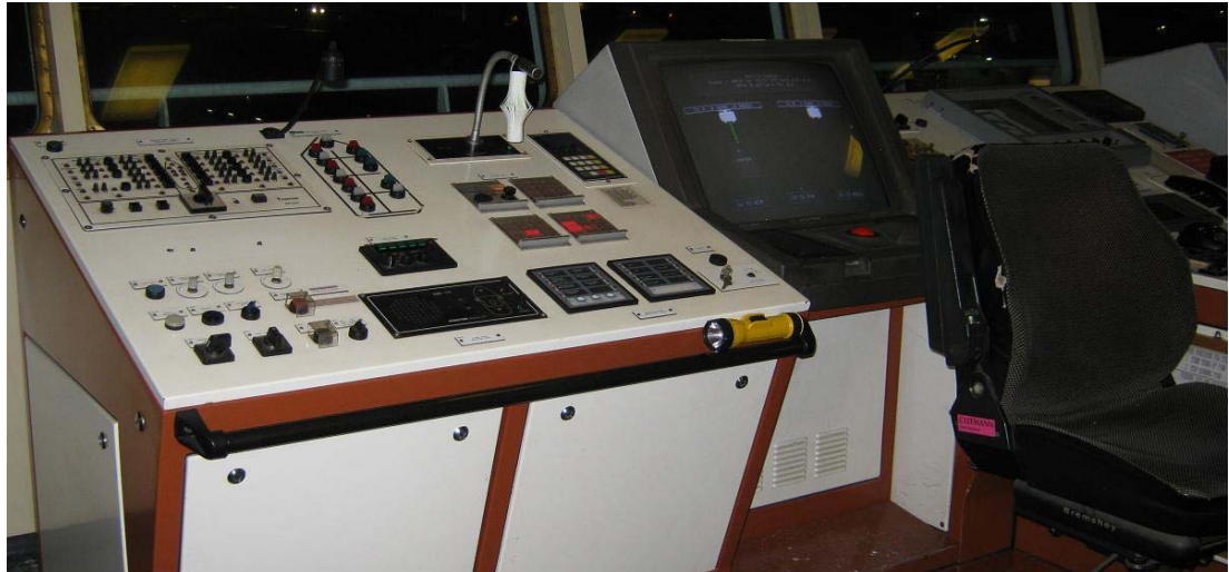
Figure 4. The general arrangement of the bridge; portside workstation, radar display, control devices and control panels in the console.
