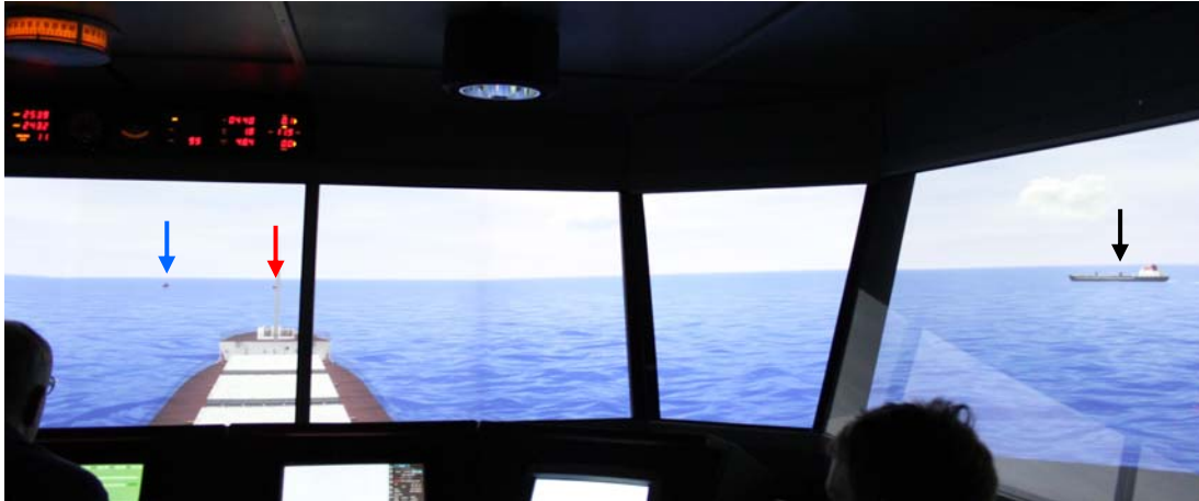
Image 7. The change of direction to the starboard starts with the rudder command “hard to starboard”. The distance to the fishing vessels is 0.58 miles. The FLORENCE is marked with a blue arrow, the MENHADEN with a red arrow, and the STELLA POLARIS with a black arrow.
