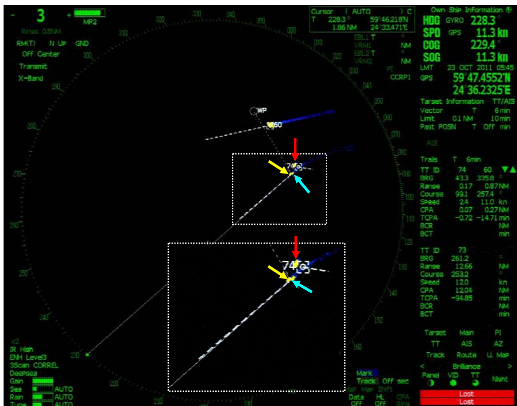
Image 14. At 04:44:56, the AMAZON's change of the course to the port has ceased (the heading, and the vectors indicating the course, are overlapping). The course of the AMAZON is 229.4°, with a speed of 11.3 knots.
