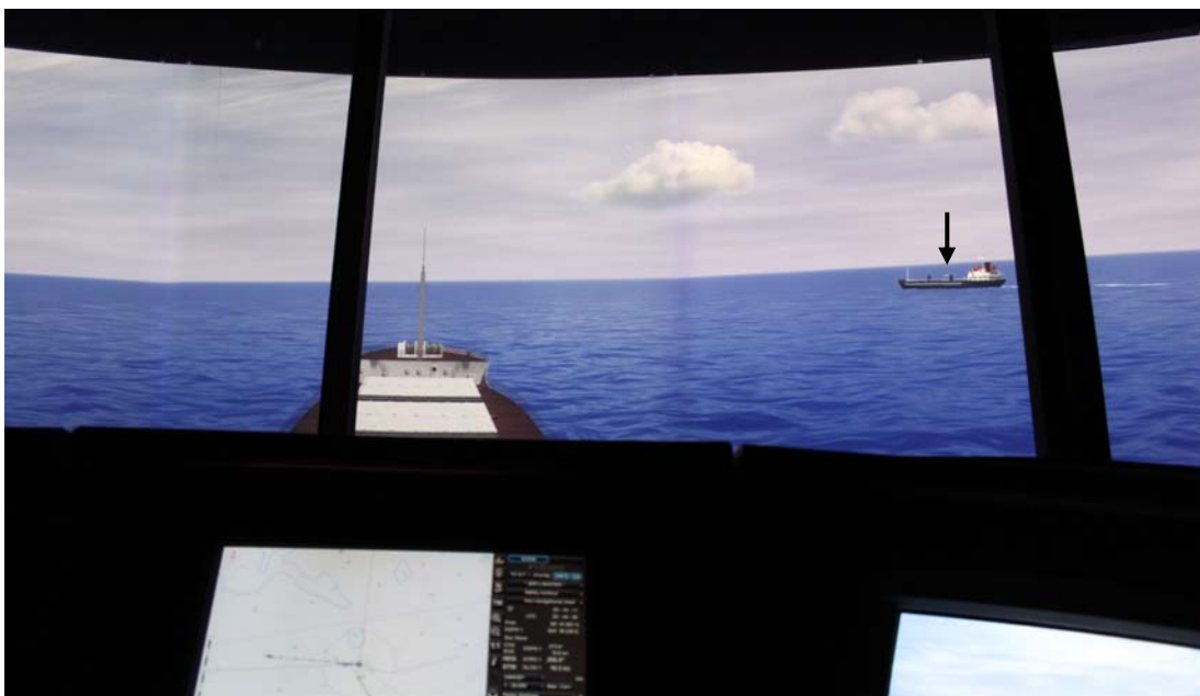
Image 10. The change of direction to the starboard is ready, and the change of direction back to the original course has been initiated a moment earlier. The fishing vessels pass from the port side, and the distance to the STELLA POLARIS (black arrow) is approximately 0.4 miles.
