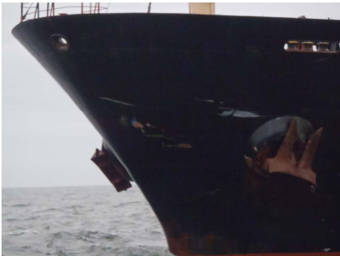
Image 17. Photograph of the bow of the AMAZON, taken while the vessel was detained in front of Hanko after the accident. Scratches and damage to the paint are visible on the port side of the bow.
