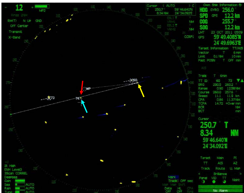
Image 2. At 04:09:34, approximately 34 minutes before the collision. The radar range is 12 miles. The OOW of the AMAZON has just begun the ARPA monitoring of the fishing vessels (number 74 on the screen) so the additional radar information is not displayed on the radar screen yet. The course of the AMAZON is 255.7° with a speed of 12.2 knots.
