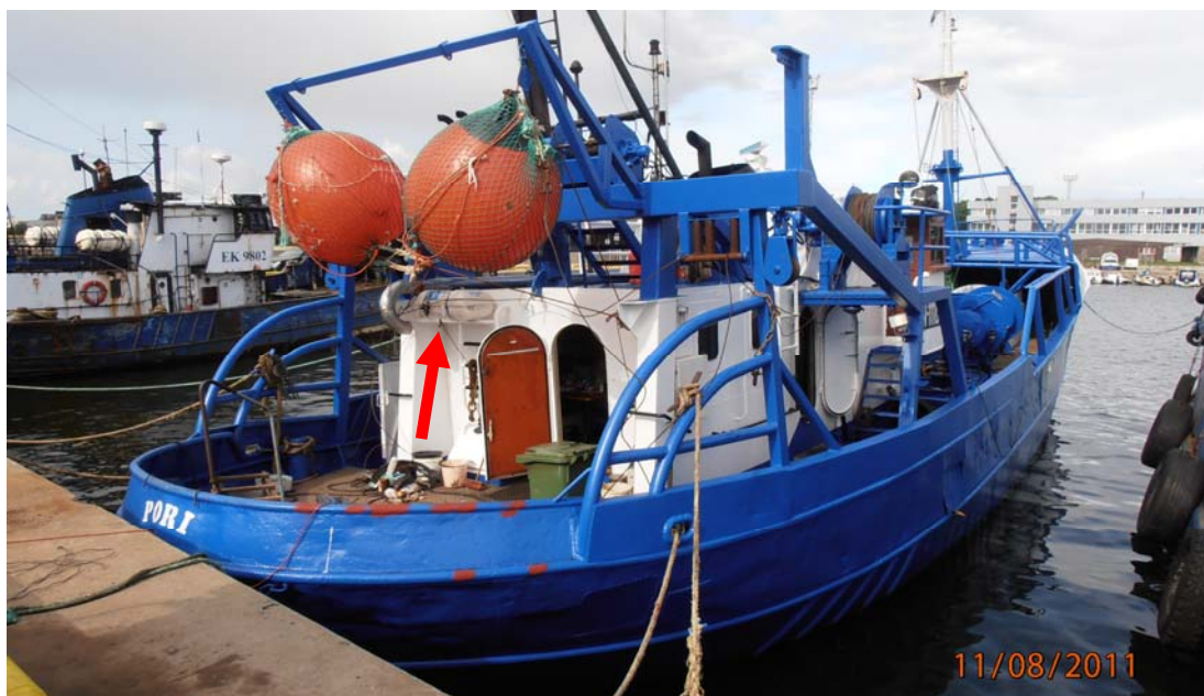
Image 16. The red arrow shows the location of the liferaft on the FLORENCE. The crew managed to escape the deckhouse through the backdoor open in the photograph. (© Kalavara)
