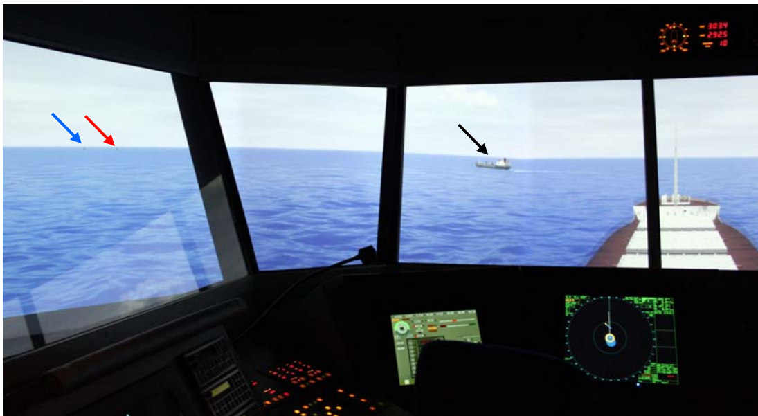
Image 6. The FLORENCE is marked with a blue arrow, the MENHADEN with a red arrow, and the STELLA POLARIS with a black arrow. Despite the turn initiated during the passing, no close-quarters situation with the STELLA POLARIS is developed because the distance to it grows during the turn.
