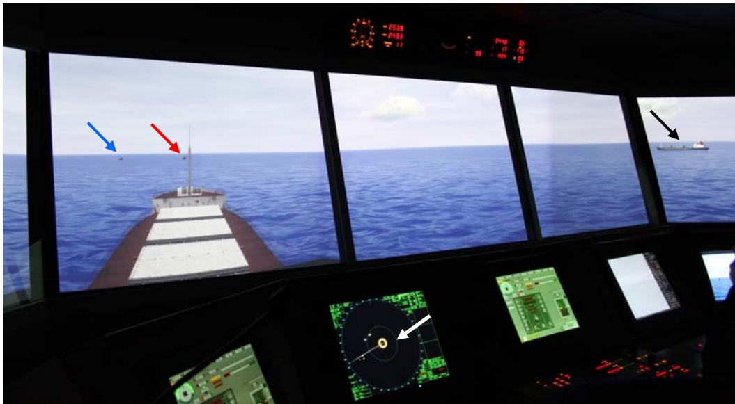
Image 3. The initiation of the change of direction is approaching. The FLORENCE is marked with a blue arrow, the MENHADEN with a red arrow, and the STELLA POLARIS with a black arrow. The VRM 48 ring on the radar that is seen in the foreground of the image is set to 0.58 miles (white arrow). The change of the course is initiated when the ring hits the displayed radar echoes of the fishing vessels. The distance to the fishing vessels in the image is approximately 0.8 miles.
