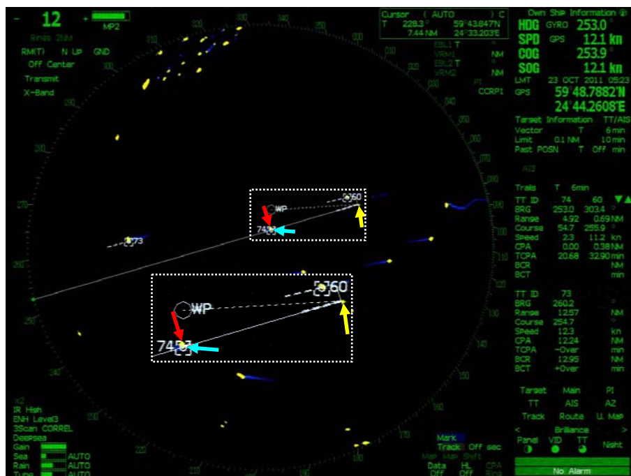
Img. 1. At 04:23:42, approximately 20 minutes before the collision. The fishing vessels are within 4.92 miles of the AMAZON in a heading of 253°. The course of the fishing vessels is 55°, and the speed 2.3 knots. The fishing vessels are directly underneath the AMAZON course vector (CPA 0 miles). TCPA 20.68 minutes. The course of the AMAZON is 253.9°, with a speed of 12.1 knots.
