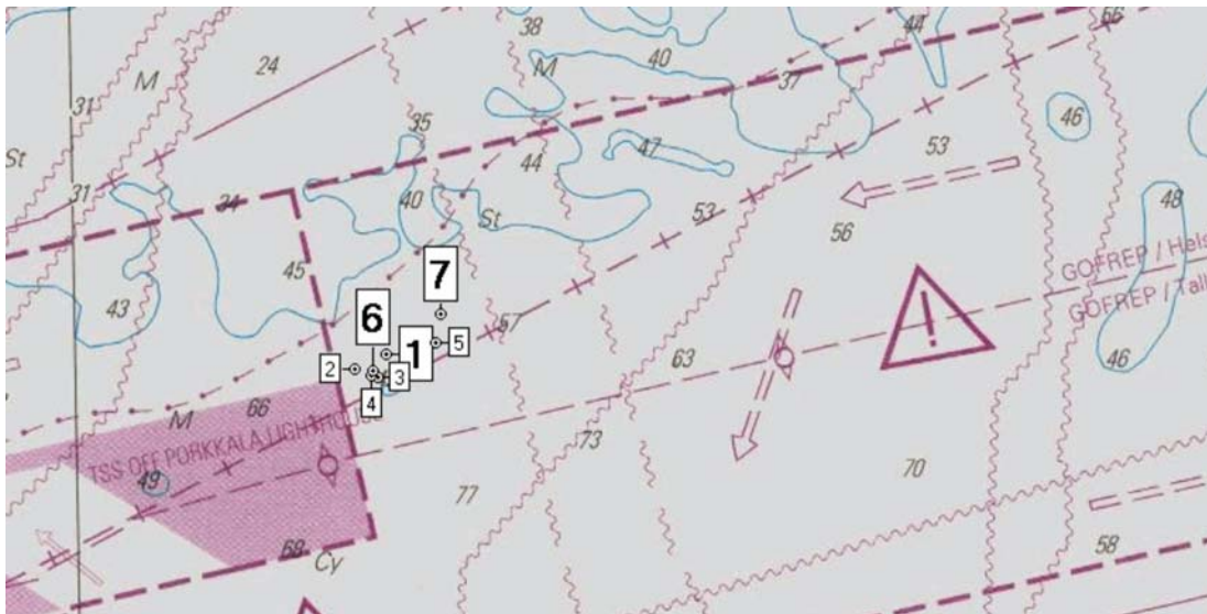
Image 20. Locations marked on the image: 1) Site of the collision, 2) where the KAUNAS observed oil, 3) where the KAUNAS observed a light and floating material, 4) where the patrol boat found waste, oil and the covers of a life raft, 5) where the patrol boat found the EPIRB of the FLORENCE, 6) the place where the FLORENCE sank, 7) where the patrol boat discovered the crew of the FLORENCE on a liferaft. The distance between the location of the sinking and the place where the life raft was discovered is approximately 0.75 nautical miles. (Map base © Finnish Transport Agency)
