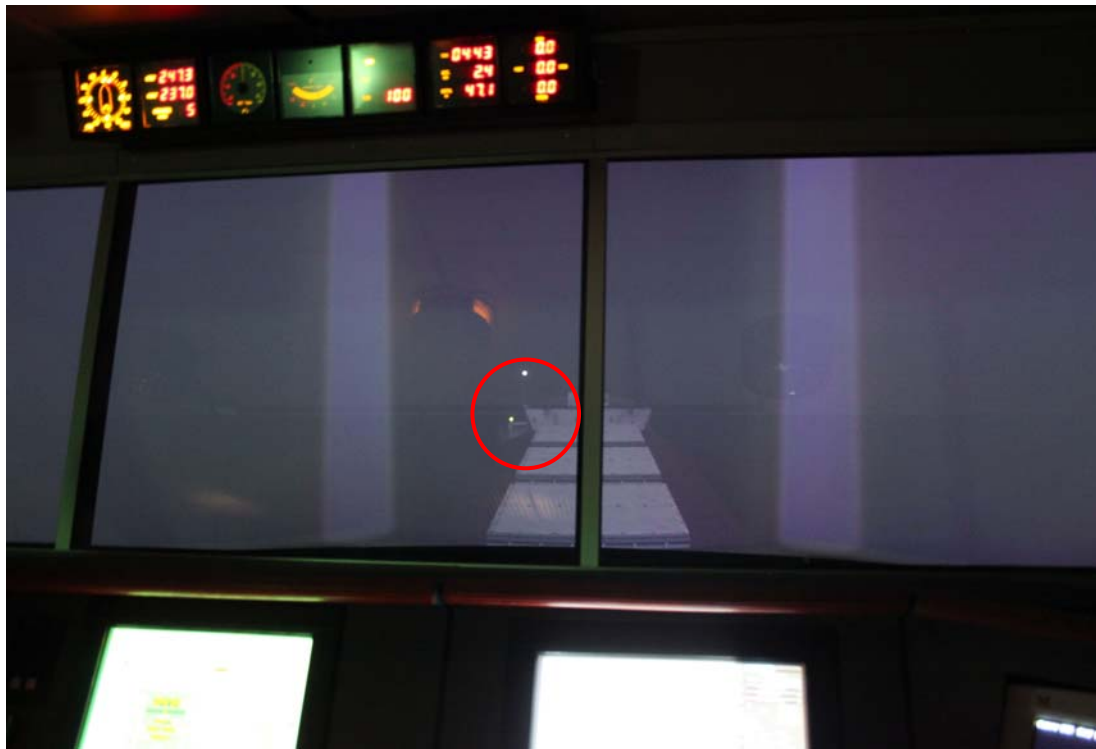
Image 2. The simulated collision is just about to happen in the fog (visibility 200m) and darkness. The FLORENCE is marked with a red circle. Its navigation lights have appeared a moment earlier. The fishing vessel's white mast-head light, green navigation light, and some of its deckhouse are visible. (During the actual accident, the vessel's cranes have probably hindered the visibility especially when looking out from the starboard side of the bridge. In that case it is possible that also the fishing vessel lights have been in a blind spot.)
