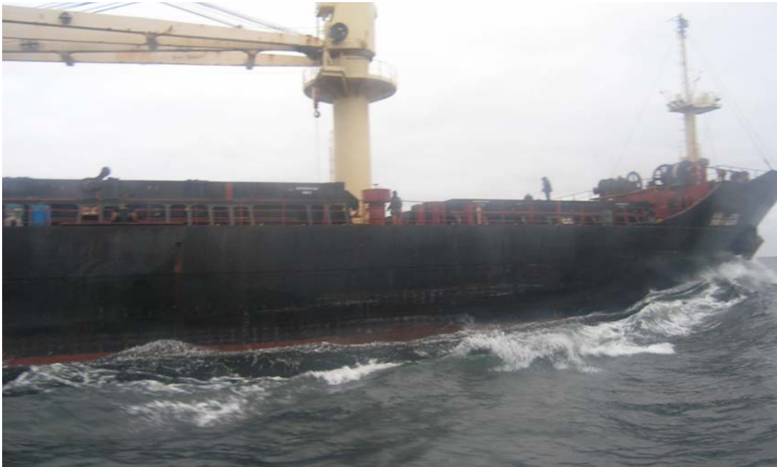
Image 27. The AMAZON moving in loaded condition. The water level rises due to the bow wave. The picture is taken on the day of the accident on 23 October, 2011, so the draught is the same as it was during the accident.
