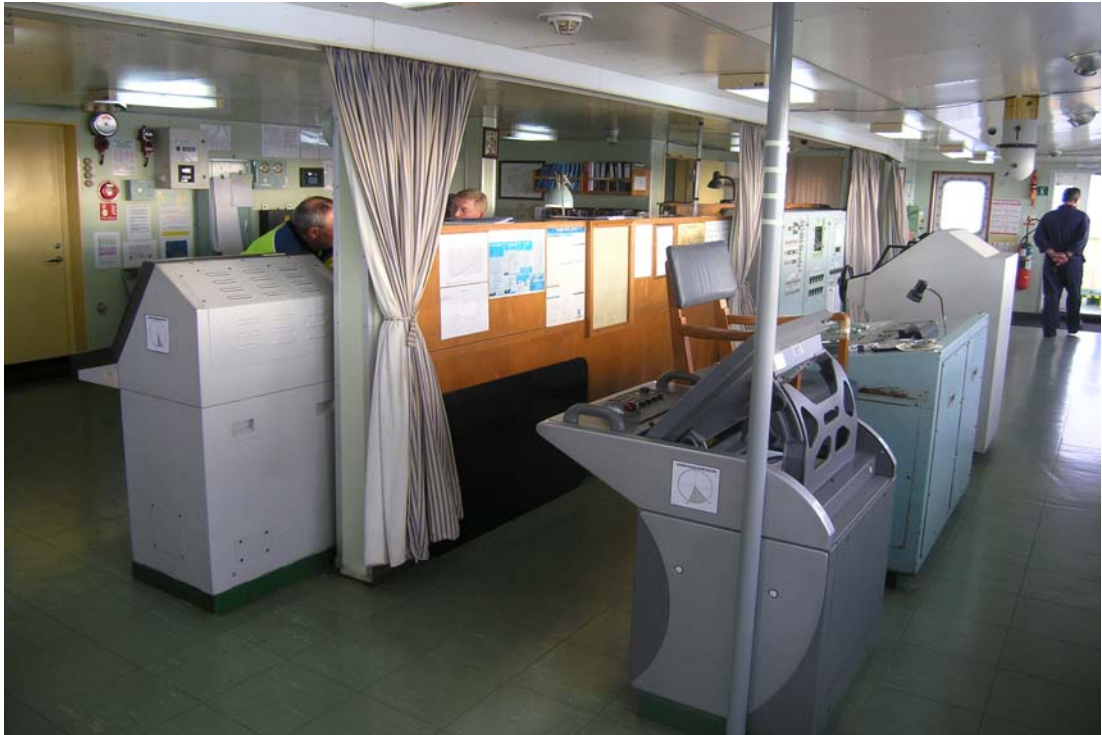
Image 5. The bridge of the AMAZON. In the dark the chart table is separated from the rest of the bridge with a curtain, as shown in the image. It obstructs the view outside from the chart table.
