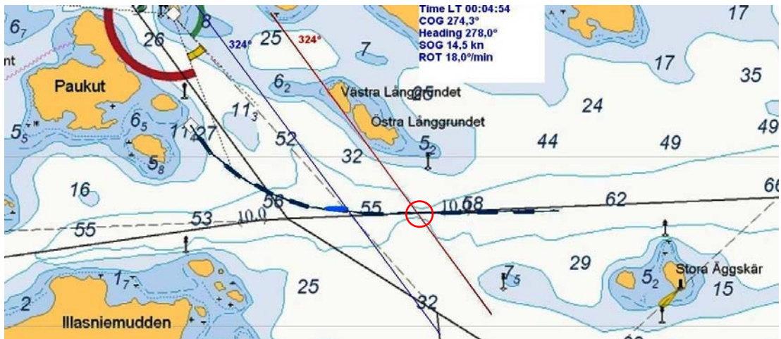
Figure 4. The ship symbols are plotted on the basis of the S-VDR recording. The red circle indicates the point where the pilot, according to his passage plan, intended to commence the turn to starboard on a COG of 269° at 14.5 knots. The pilot said that he set the autopilot heading to 300°. As per the VDR recording the heading at the position of the light blue ship symbol was 278°. The vessel continued to move in an almost straight line with a COG of 272° for 67 seconds after the pilot, according to his account, changed the heading. The Rönnggrund sector light changes from green to white. The distance between the blue and the red ship symbols is 0.27 NM and the change in heading at that time is 9°. There is a delay in the onset of the turn, which can partially be explained by the fact that the vessel only begins to turn 80 metres after receiving the steering input. (Chart: The Finnish Transport Agency, presented using Uusi Loisto programme)
