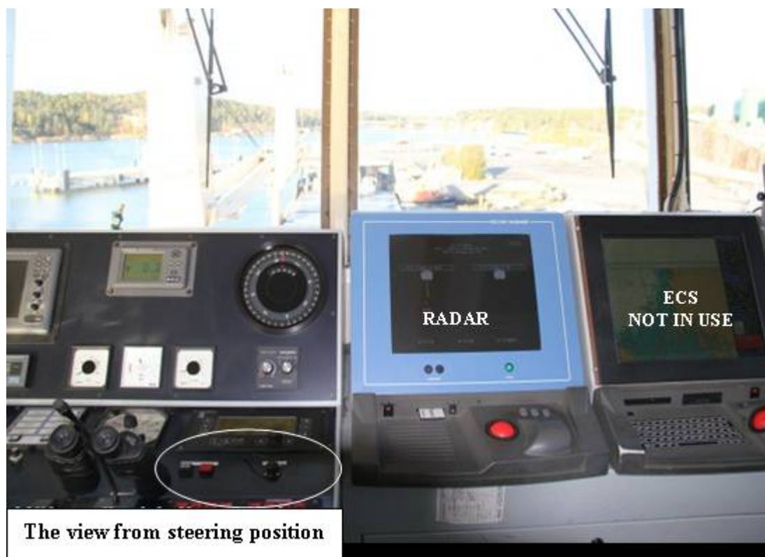
Figure 9. The pilot's steering position. The white ellipse shows the Pilotstar D autopilot.
