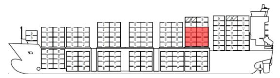
Figure 2. A layout drawing of the cargo spaces on M/S LINDA. The red rectangle indicates the location of the fallen container stack on the outermost bay on the port side of the vessel. (© Oy Langh Ship Ab)
