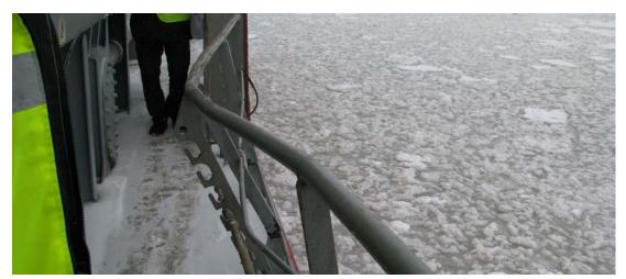
Figure 5. The railing damaged by the fallen container stack on the port side of the vessel.
