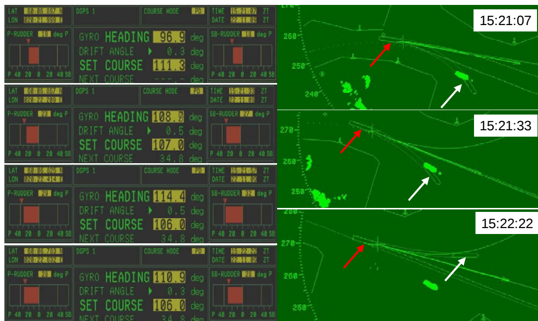
Figure 8. Large rudder angles used in the counter rudder after a turn to starboard commenced at 15:20 (Figure 7) shown on the conning-display (to the left) and corresponding picture of the radar display (to the right); the rudders are turned to port: BB rudder angle on the left and SB rudder angle on the right. In the radar pictures the position estimated by the predictor after a minute has been marked with a white arrow and the vessel's position at that particular moment with a red arrow. The green radar echo close to the white arrow is the M/S FJÄRDVÄGEN.
