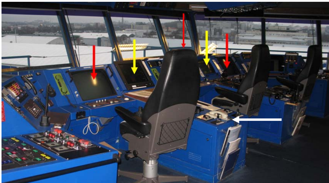
Figure 2. View from the navigating bridge, the vessel's steering positions. The picture was taken on 24 November 2009 in Turku. The red arrows point to the radar displays (one of them is hidden behind the chair) and the yellow arrows indicate the conning displays. The route pilot's chair (main steering) is in the middle, the OOW's chair (monitoring navigator) is to the right and to the left is the Master's chair. The white arrow indicates the control console of the hydraulic accumulators of the steering gear, the levers on the right and left side.
