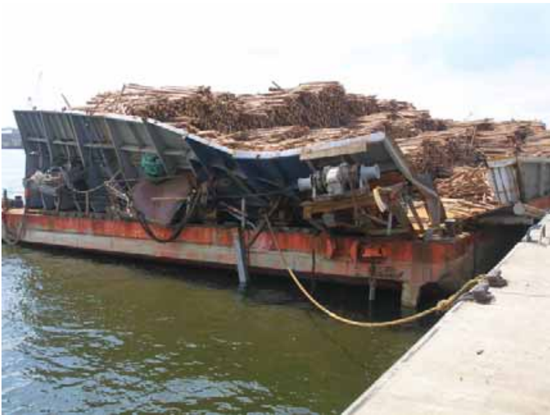
Figure 10. Damage to the aft of the barge CARRIER. (Figure Sjöfartsverket.se)
