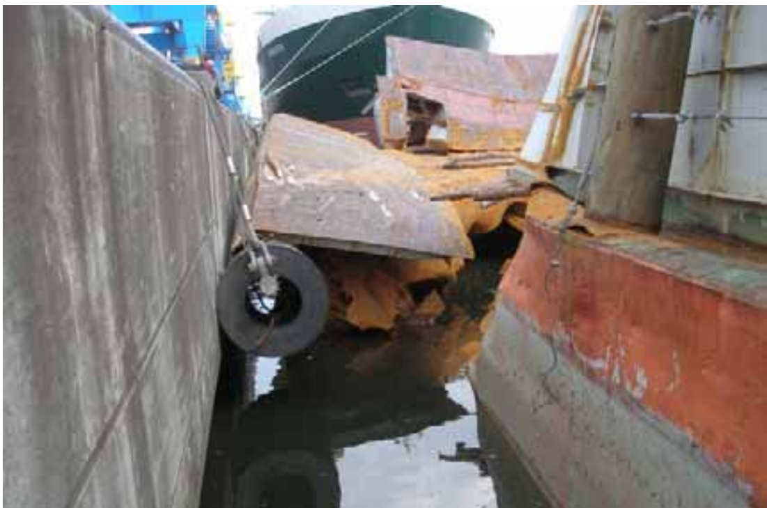
Figure 9. Damage to the side of the barge CARRIER.
