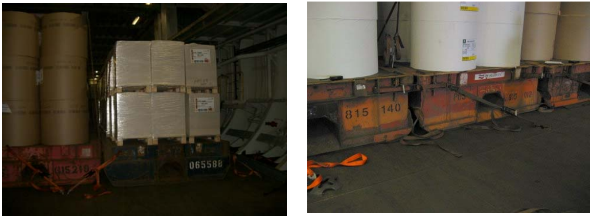
Fig. 6 The photo at the left shows roll-trailer 625 219 stowed on the Tank Top on board Finnforest and only secured with a half cross at the front of the unit. The Photo at the right shows roll-trailers on the Main Deck secured with a half cross plus one horizontal lashing.
