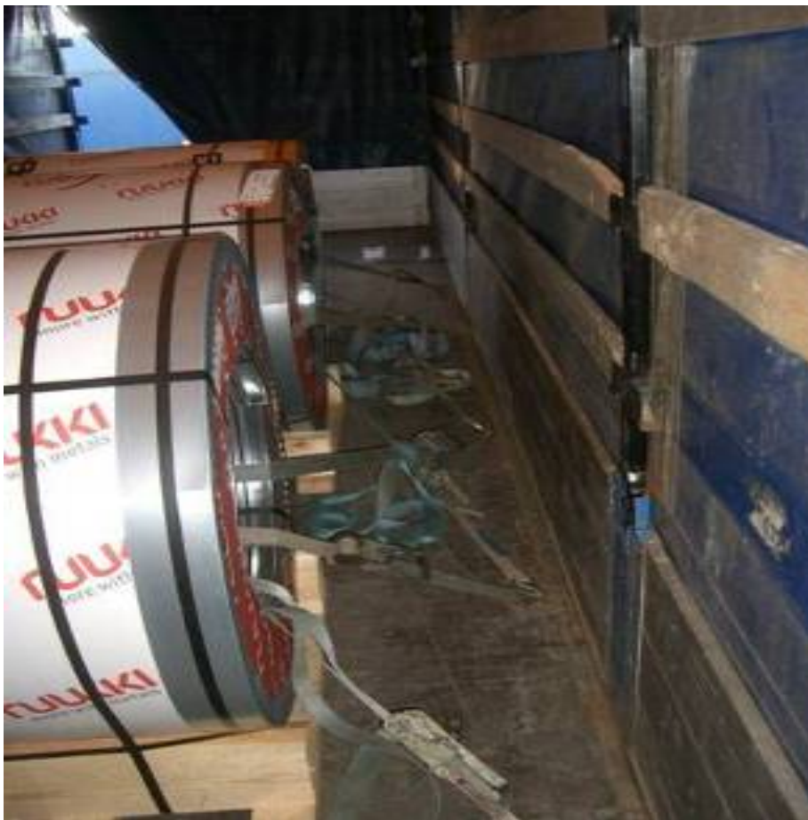
Fig 14 6-tonnes steel coils from Rautaruukki loaded on semi-trailer in Finnforest. These are secured in accordance with the company's instructions.
