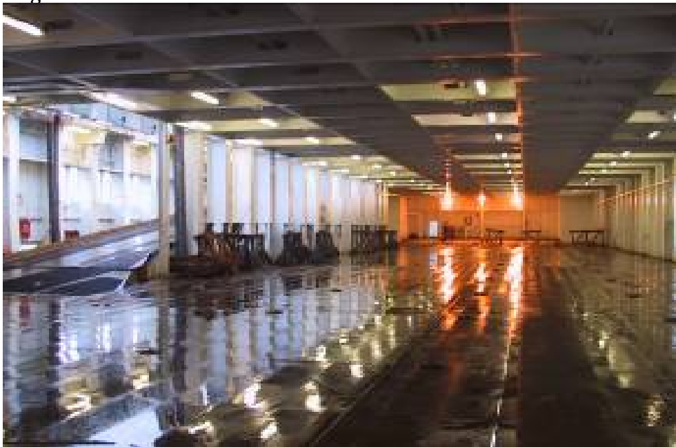
Fig. 3 The above photo taken on board the sister ship M/V Finnforest in Helsingfors in December 2006 shows the collection of water on the Upper Deck following rain.
