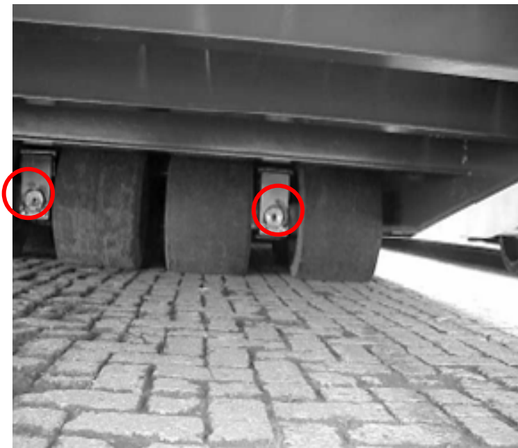
Fig. 42 Tipping points at the boggie end of a normal 40 ft. roll-trailer.
