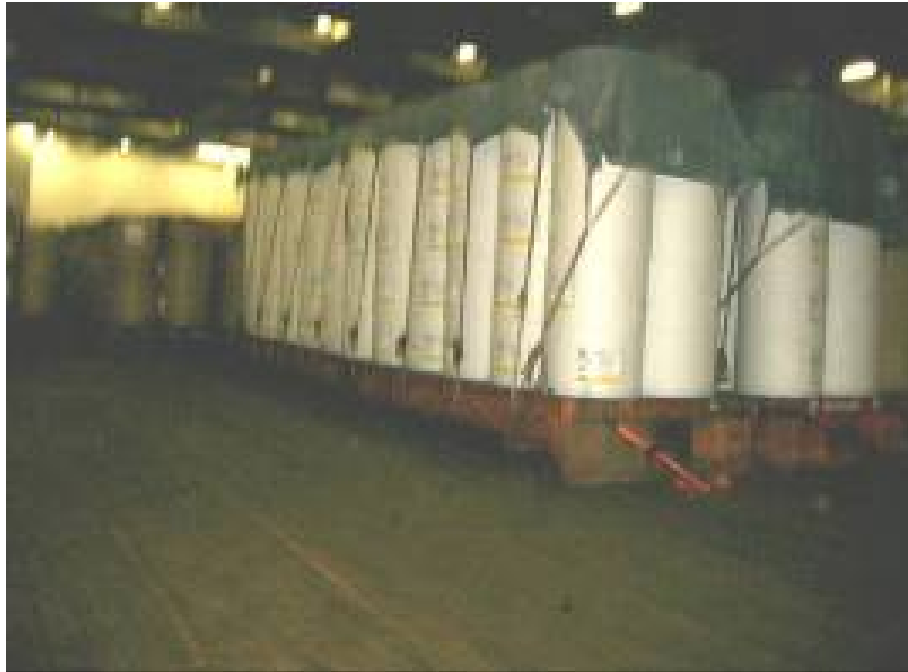
Fig. 46 Roll-trailers stowed on the Main Deck on board Finnforest. The load is secured with WisaFix hoods.
