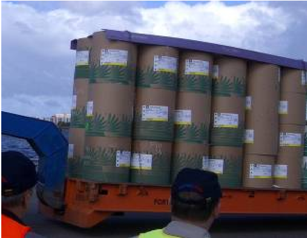
Fig. 8 Paper reels on a roll-trailer during discharge of cargo from M/V Antares at Rostock in September 2004. Two chains per long corner protection secure this cargo.
