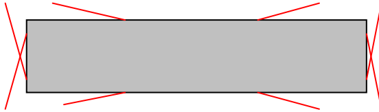
Fig. 4 Sketch showing how the Master considers the lashings should be applied on a lane stowed roll-trailer, as seen from above.
