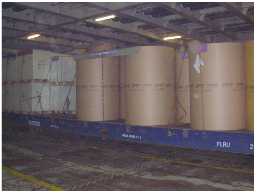
Fig. 10 Securing of large diameter reels on board the sistership Finnforest. A lashing has been placed over the midpoint of a long corner protection which holds two reels. At the left are palletted goods in the form of sheet paper. Photo taken during a visit by SHK in September 2007.
