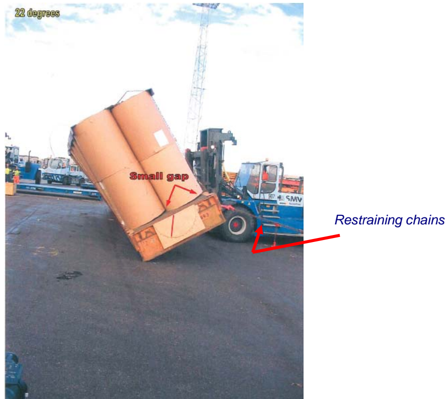
Fig. 43 Heeling tests showing that roll-trailers with high load are very likely to tip.
