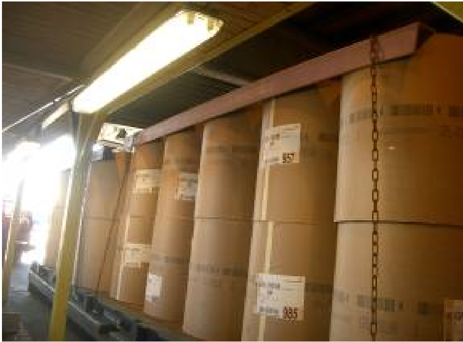
Fig. 9 Paper reels stowed on a cargo transport unit in the Helsinki terminal, a cargo section 5.25 m long secured with corner protection and two chains. Photo taken during visit by SHK in September 2007.
