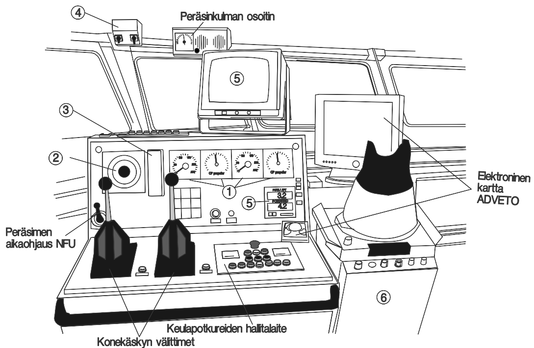
Figure 8. The texts in the figure indicate systems needed in port manoeuvring.
