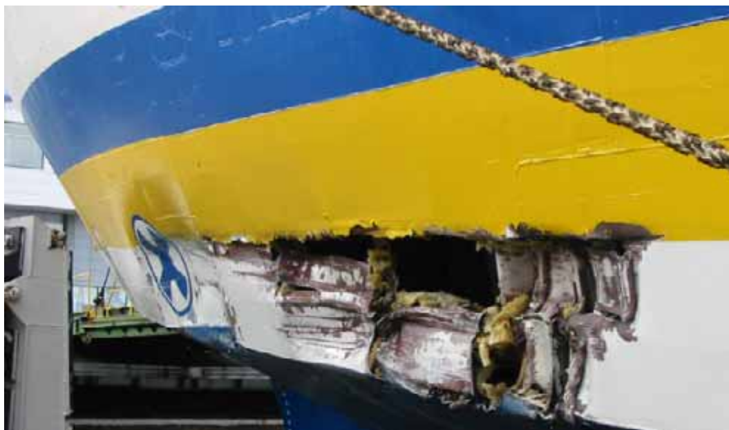
Figure 20. The NORDLANDIA's damage on the port side bow of the vessel. The damage was caused by the collision with the fender of the quay. The shock absorbing part of a similar but an intact fender can be seen to the left in the figure.
