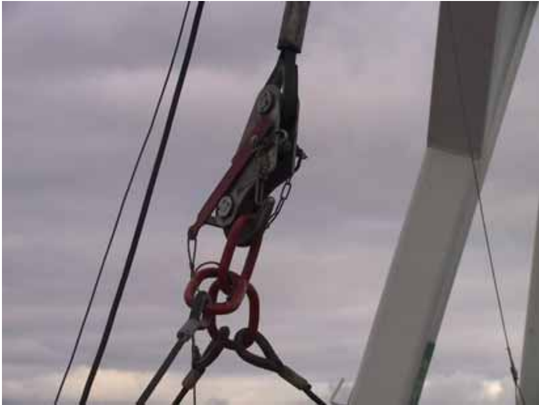
Figure 4. The hook of the boat in the accident, where the bolt used as the security pin is in place. The release wire goes downwards from the release lever. The charging cable of the battery and its support wire are on the left.
