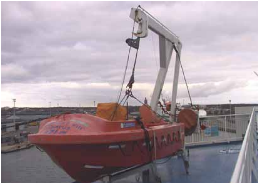
Figure 2. The MOB boat, the hoisting davit and the hoisting hook. In addition to the hoisting wire, also the charging cable of the battery and its support wire came from the davit.
