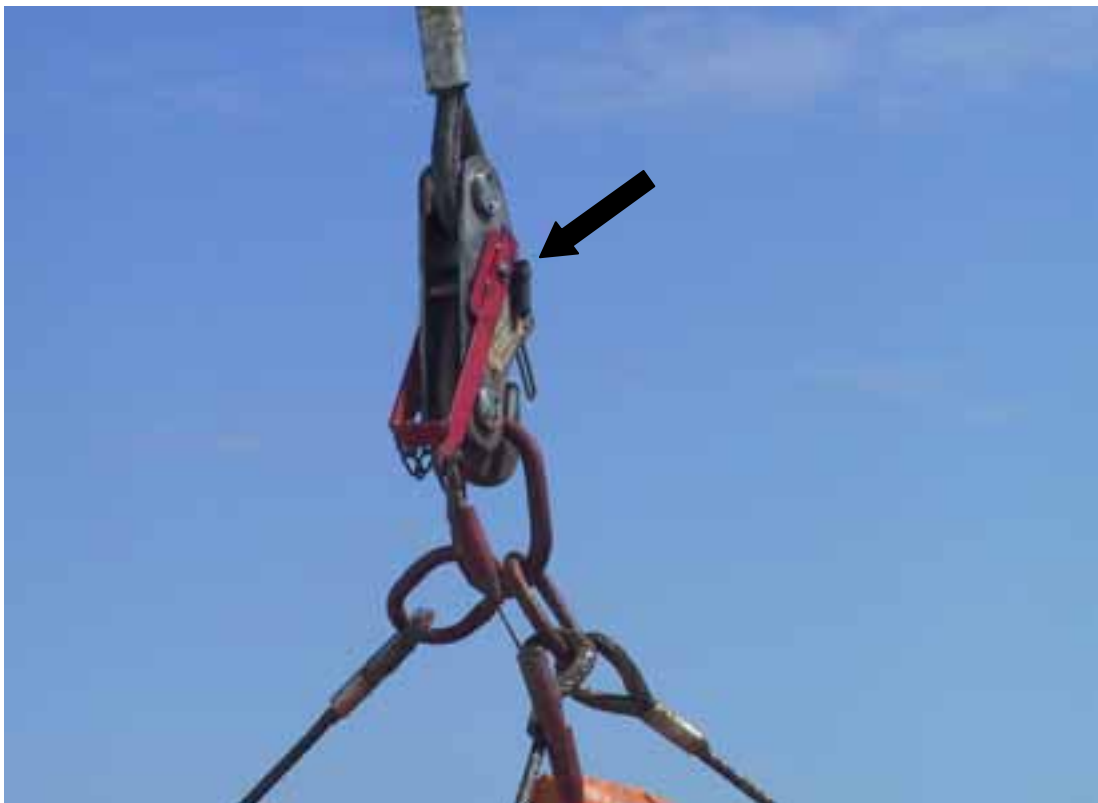
Figure 6. The hoisting hook mechanism of the corresponding boat of the sister vessel, where the arrow points to the original security pin. The red plastic cones around the release wire are here correctly, i.e., with the tapered end downwards. In the hook involved in the accident, the tapered end pointed upwards, which made the releasing slightly more difficult.
