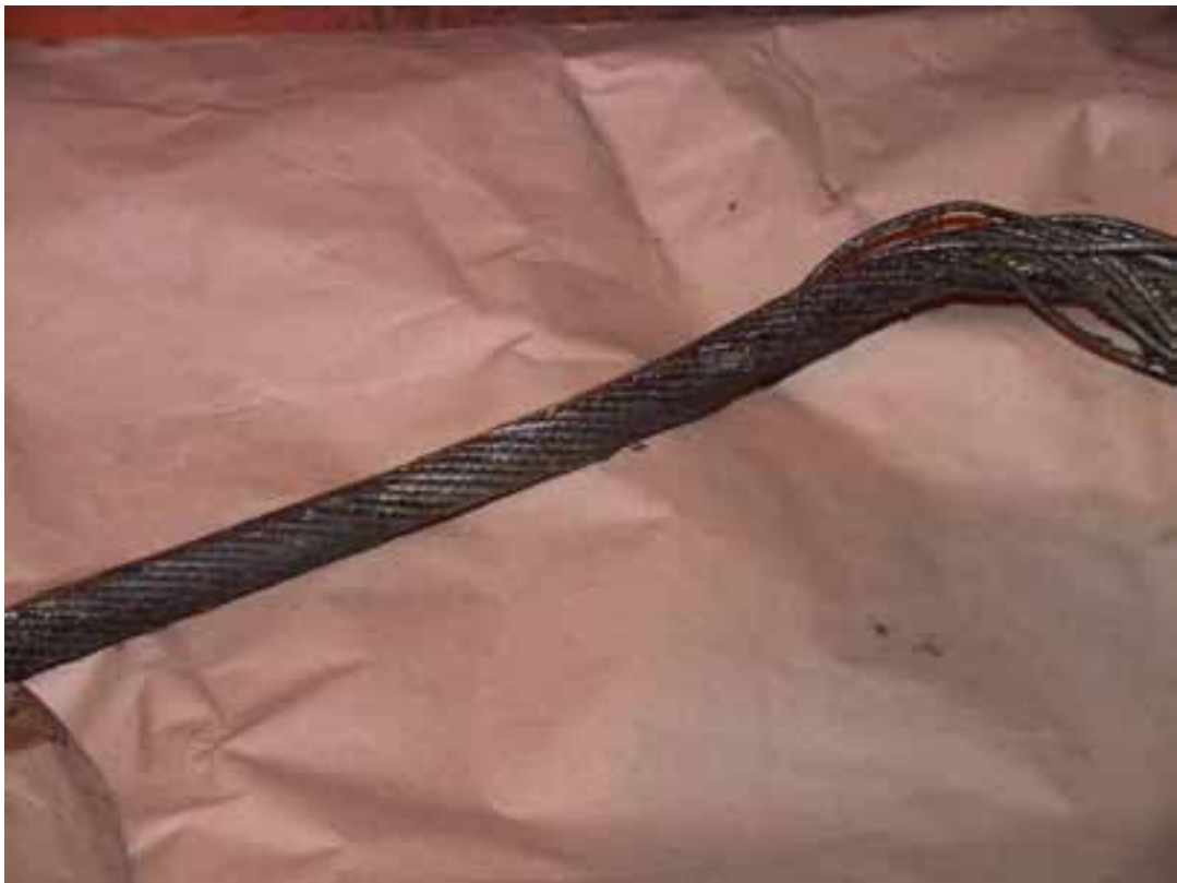
Figure 7. The fall wire; in the middle part there can be seen traces of the talurite clamp (mechanical splice).
