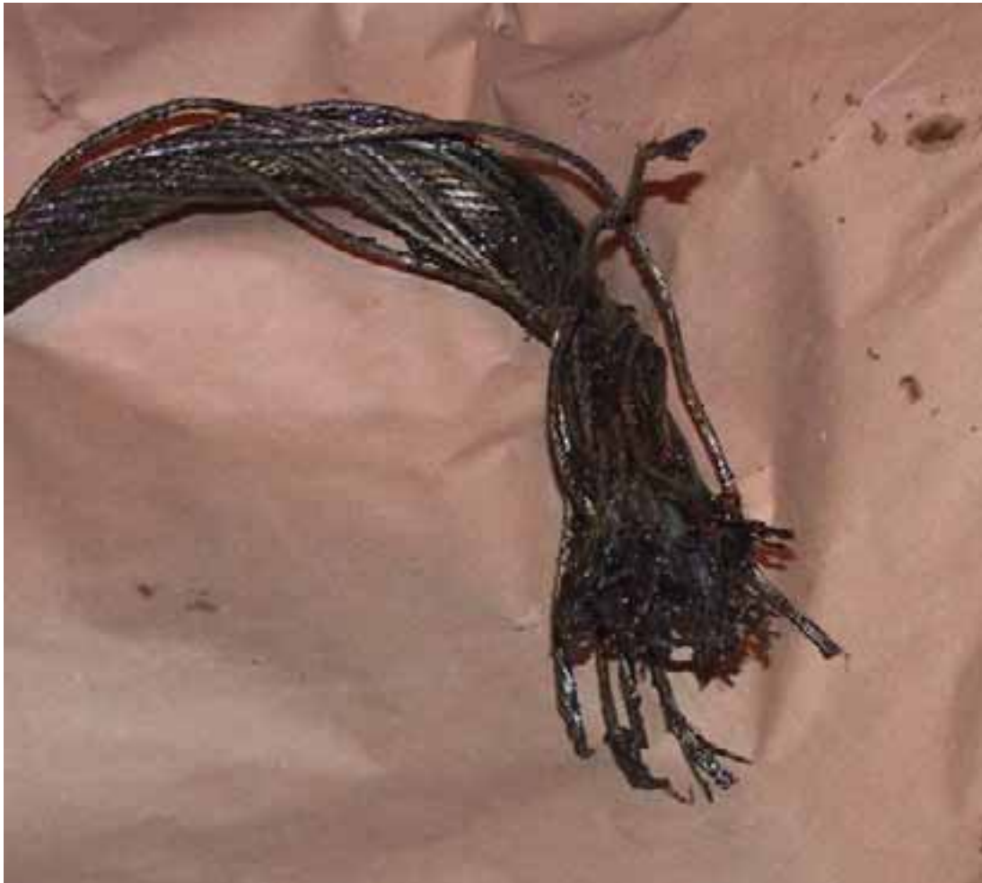
Figure 8. The ends of the strands of the fall wire are not stretched, instead they are even.
