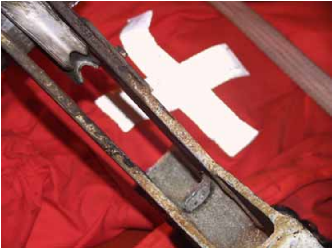
Figure 6. The position of the fall wire's eye and talurite and the guide hole for the wire.
