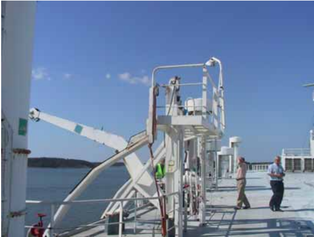
Figure 2. The rigging station for the MOB boat.
