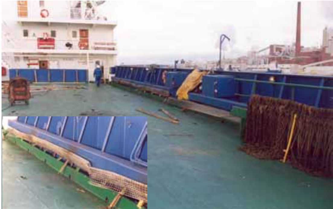
Figure 14. The damaged cowbridge on TRADEN's weather deck.
