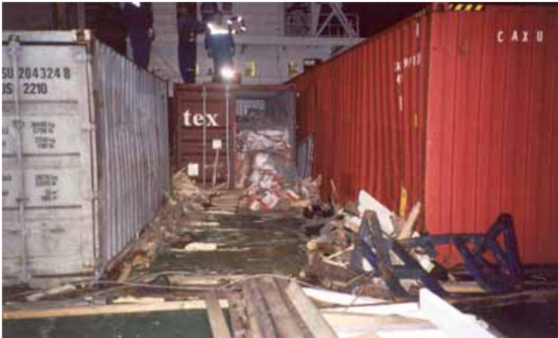
Figure 16. Damaged containers on the weather deck.
