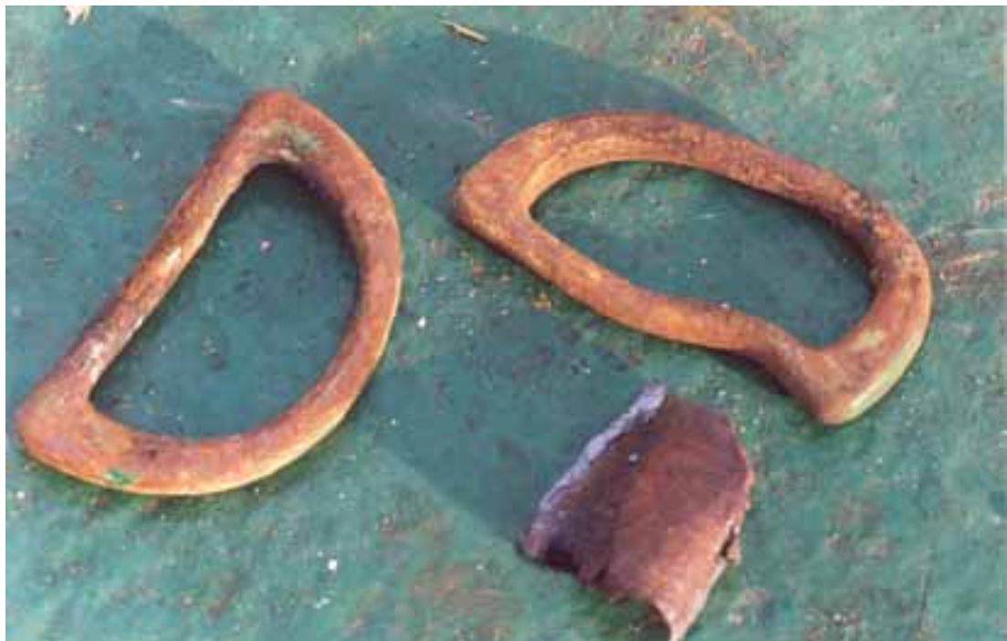
Figure 15. D-rings in poor condition on TRADEN's weather deck.
