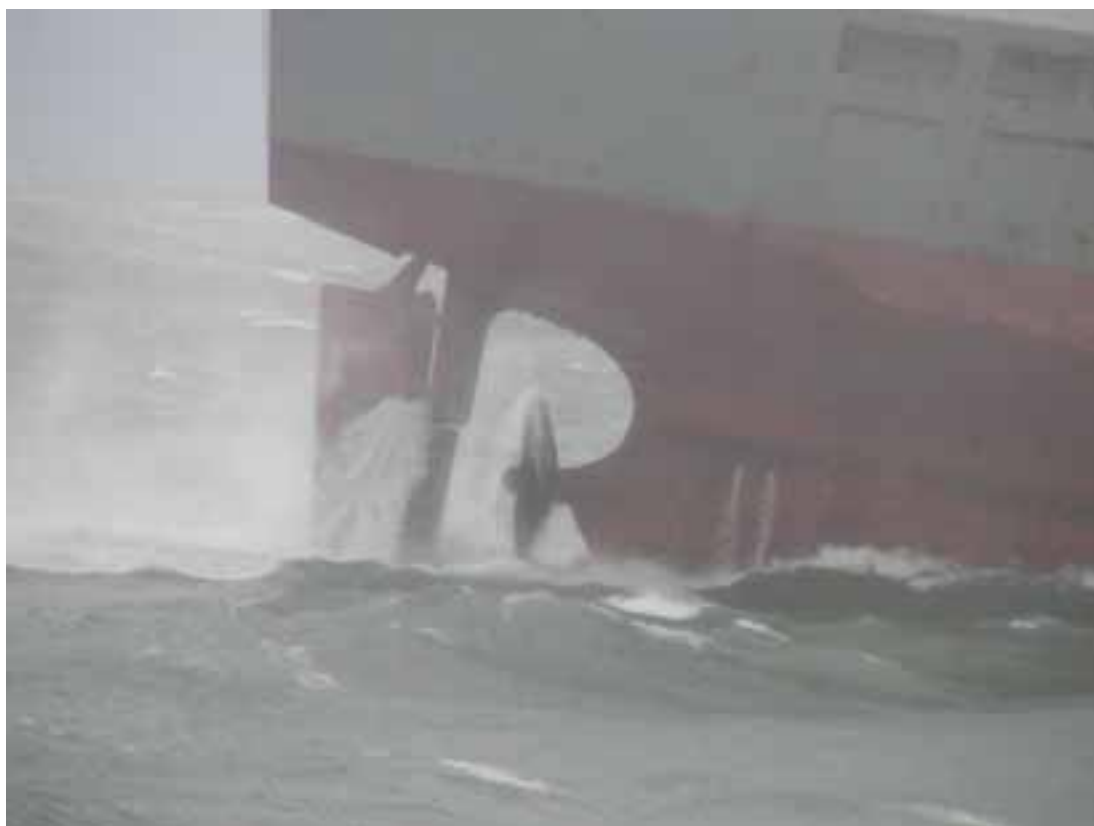
Figure 5. IRAN SARBAZ at anchor in the waves. The propeller was fully exposed at times. The rudder was turned to port. (Photo by the Finnish Coast Guard)
