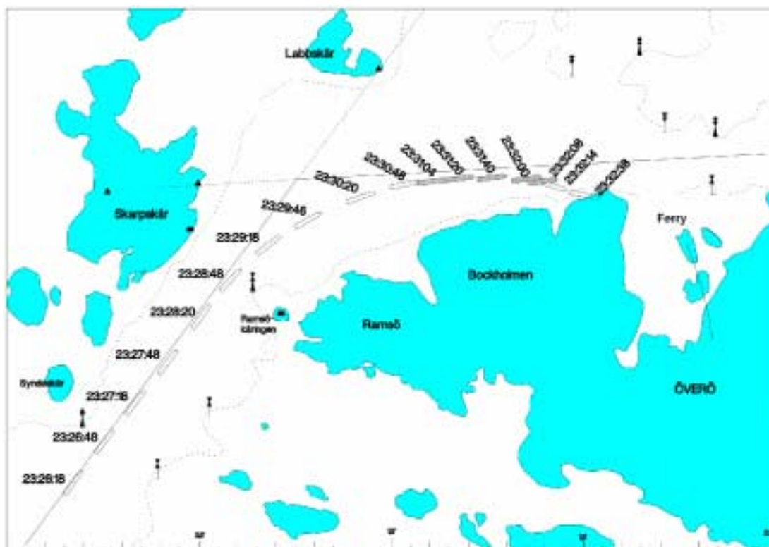
Figure 27. Data recorded by the ANS during the Skarpskär turn. The compass heading was jammed between 23:31:02 and 23:32:08.
