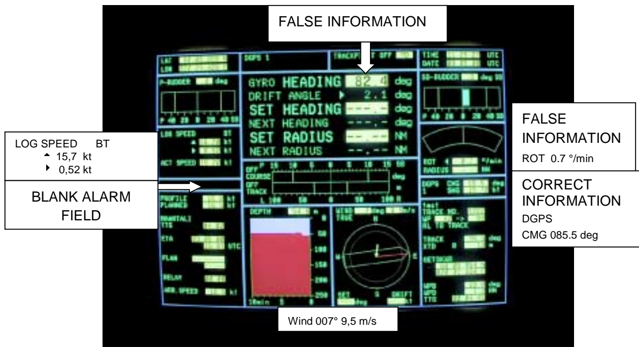
Figure 20. 15 seconds after the jamming of the compass. The picture corresponds to the situation in radar image 19.
