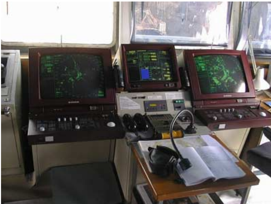
Figure 3. Integrated navigation and steering console of ms FINNFELLOW.
