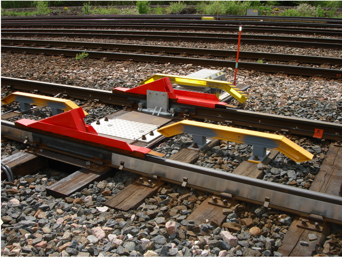
Figure 20. Emergency stop turned on the track.
