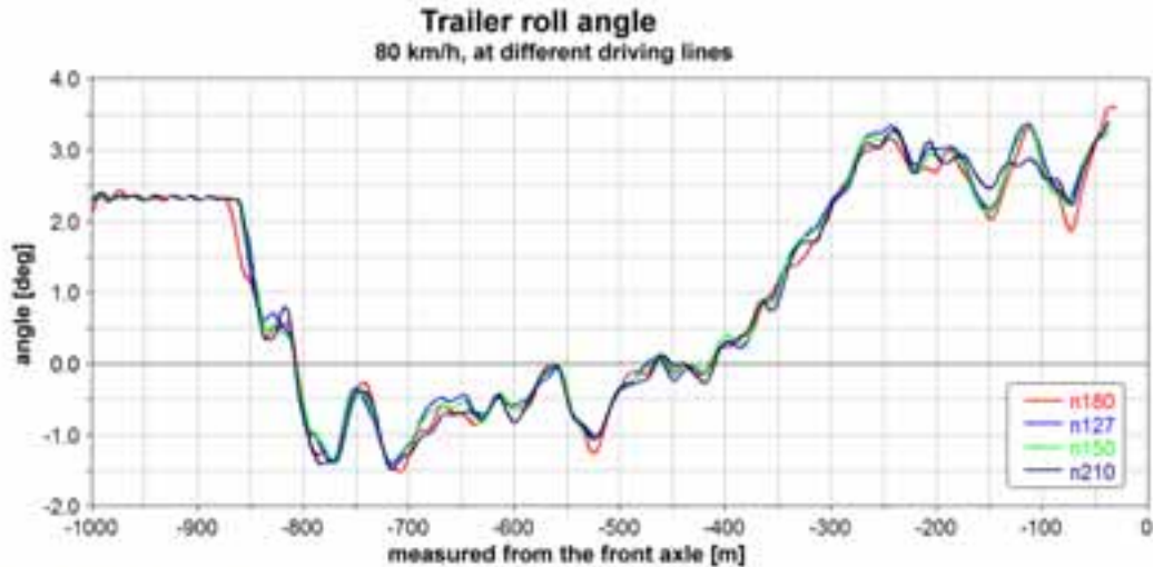
Figure 19. The trailer frame's roll in different driving lines. Positive angle = roll to the right. Coordinate 0 = point of collision.
