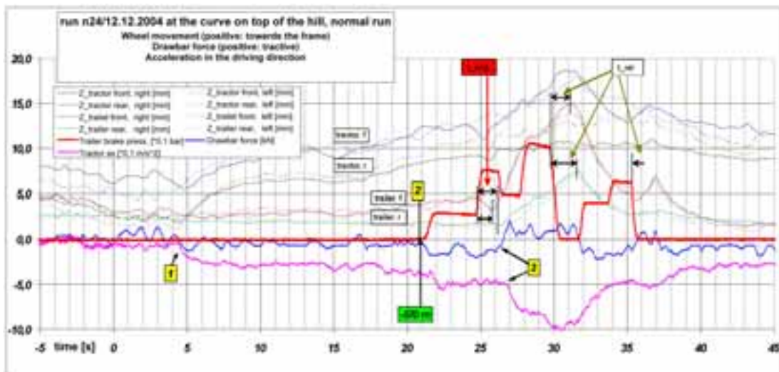
Figure 13. Measured brake lags and forces on the drawbar during test runs on 12.12.2004.
