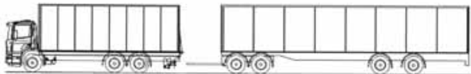
Figure 35. Tailored module trailer with a fixed front bogie. (This was the type of the vehicle in the accident.)
