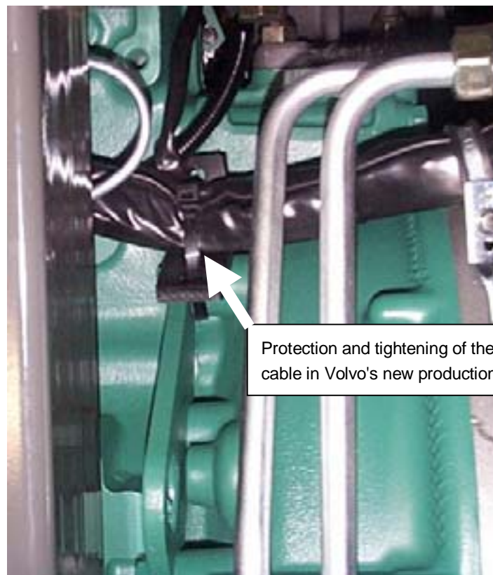
Figure 3. The tightening of the cable in Volvo's new production. The hoist bracket is below the tightened cable. (Photo : Volvo Ab)
