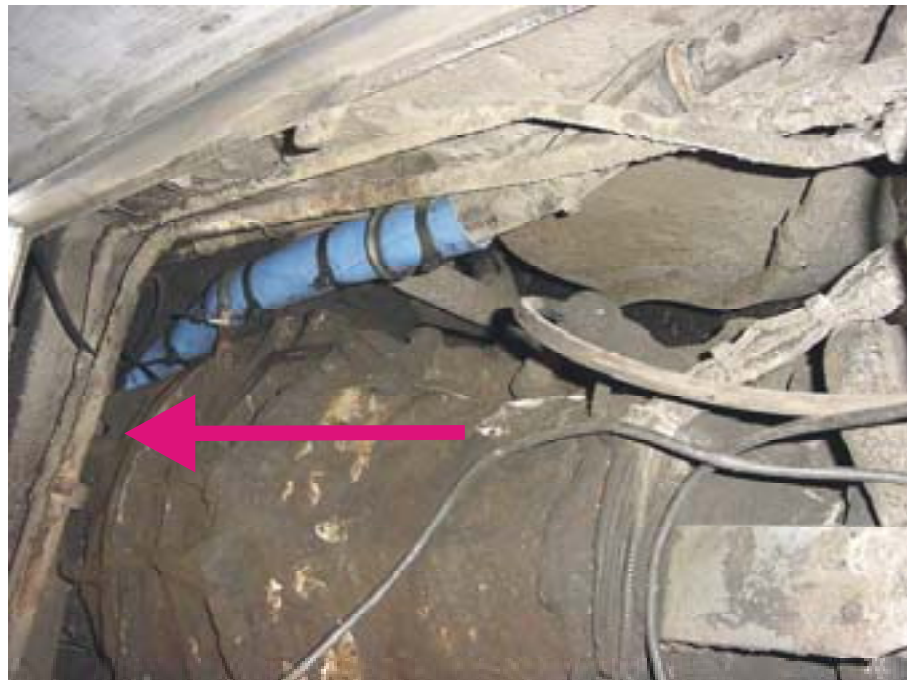
Figure 2. Protection and tightening of the battery cable at the repair shop. The wiring loom has been protected from abrasion with protective tubing and supported well. (Photo : Oy Pohjolan Liikenne Ab)
